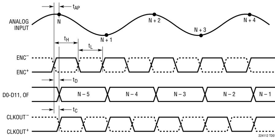
**Full-Rate CMOS Output Mode Timing**
