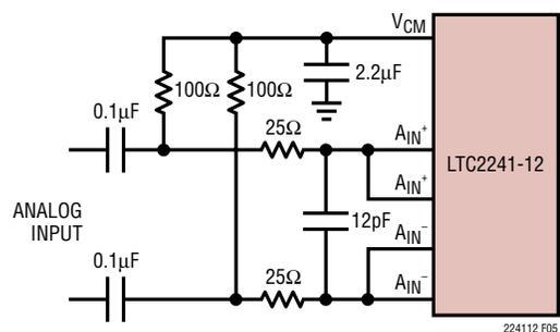
Figure 5. Capacitively-Coupled Drive
