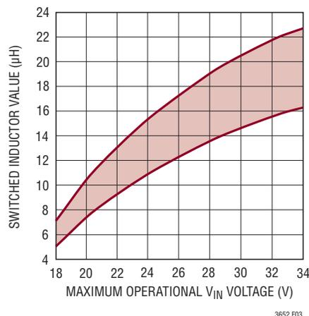
Figure 3. 14.4V at 1.5A Switched Inductor Values
