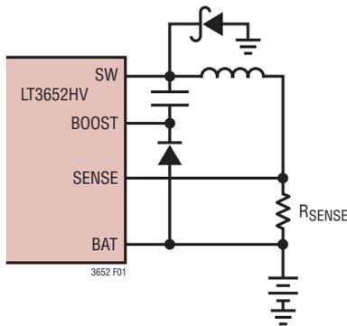
Figure 1. Programming Maximum Charge Current Using  $R_{SENSE}$
