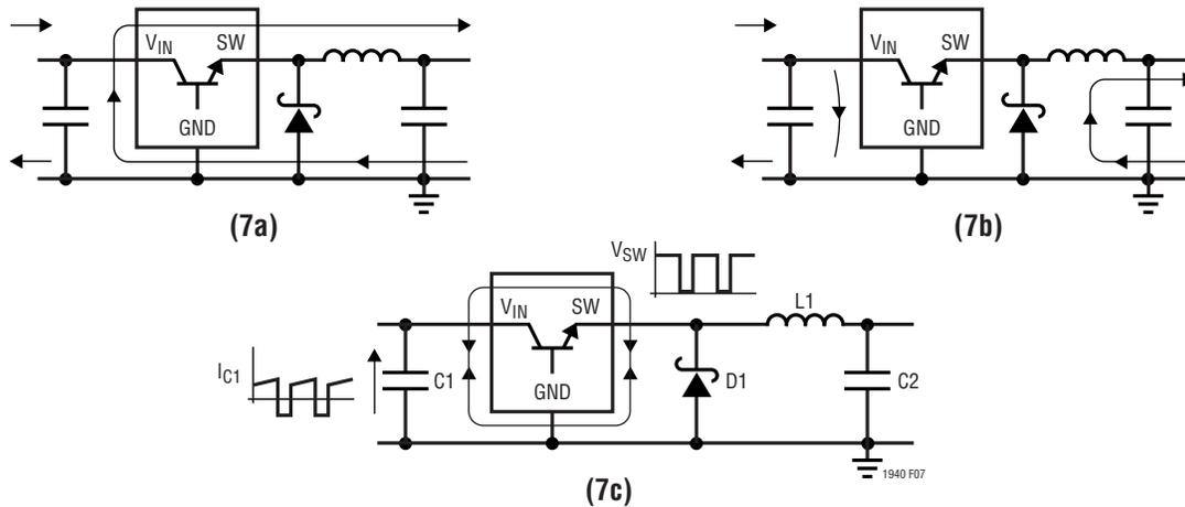
**Figure 7. Subtracting the Current when the Switch is ON (a) From the Current when the Switch is OFF (b) Reveals the Path of the High Frequency Switching Current (c) Keep This Loop Small. The Voltage on the SW and BOOST Nodes will also be Switched; Keep these Nodes as Small as Possible. Finally, Make Sure the Circuit is Shielded with a Local Ground Plane.**
