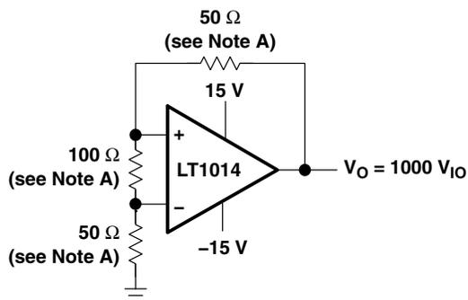
NOTE A: Resistors must have low thermoelectric potential.
