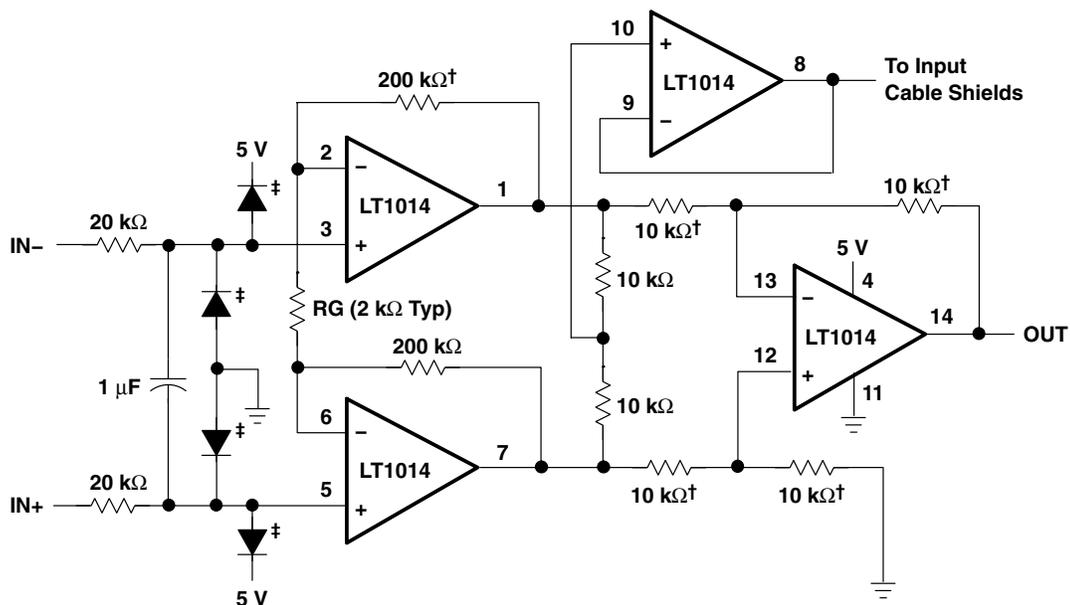
† † 1% film resistor. Match 10-kΩ resistors 0.05%.
