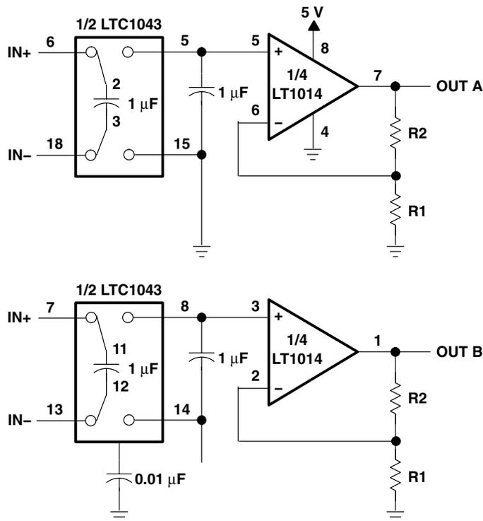
NOTE A:  $V_{IO} = 150 \mu\text{V}$ ,  $A_{VD} = (R1/R2) + 1$ ,  $\text{CMRR} = 120 \text{ dB}$ ,  $V_{ICR} = 0 \text{ to } 5 \text{ V}$
