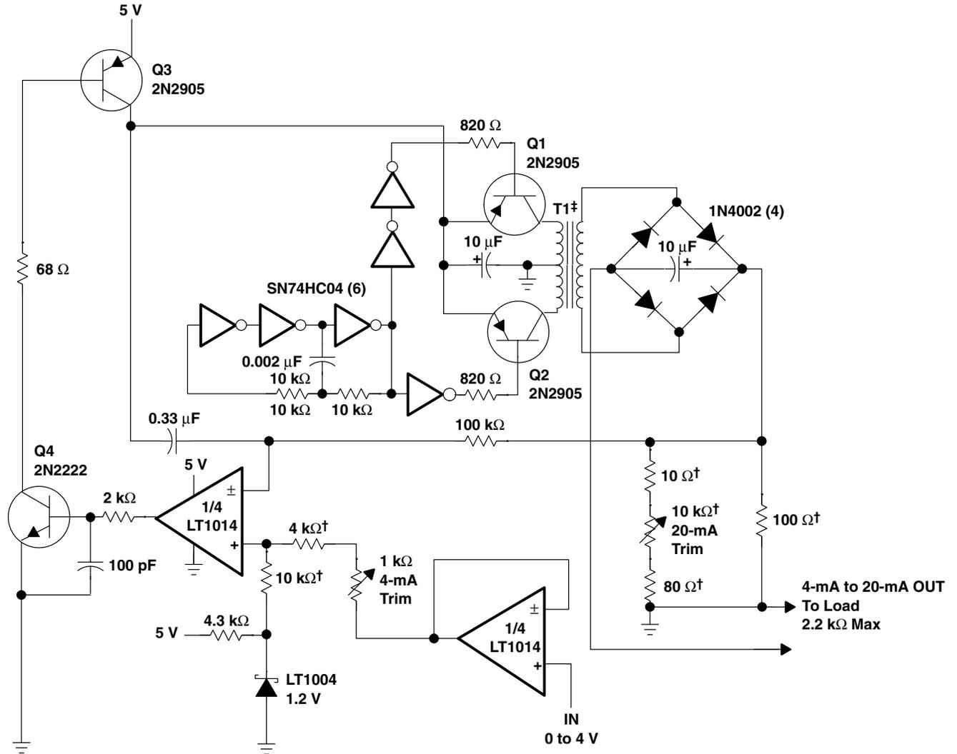
† 1% film resistor. Match 10-kΩ resistors 0.05%.
