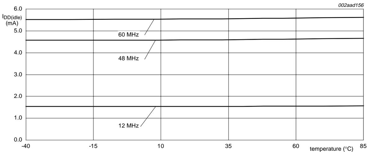
Test conditions: Idle mode entered executing code from on-chip flash; PCLK = CCLK<sub>4</sub>; core voltage 1.8 V; all peripherals disabled.
