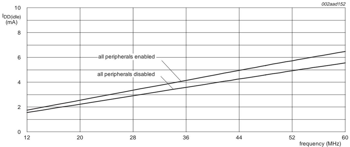
Test conditions: Idle mode entered executing code from on-chip flash; PCLK = CCLK<sub>4</sub>;
