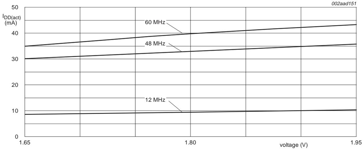
Test conditions: Active mode entered executing code from on-chip flash; PCLK = CCLK<sub>4</sub>;
