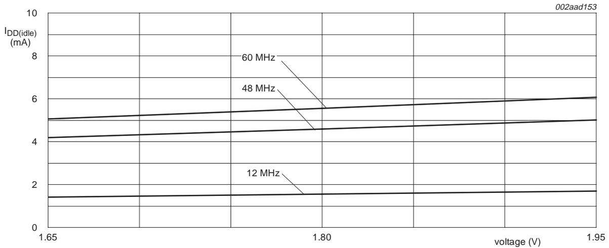
Test conditions: Idle mode entered executing code from on-chip flash; PCLK =  $CCLK/4$ ;
