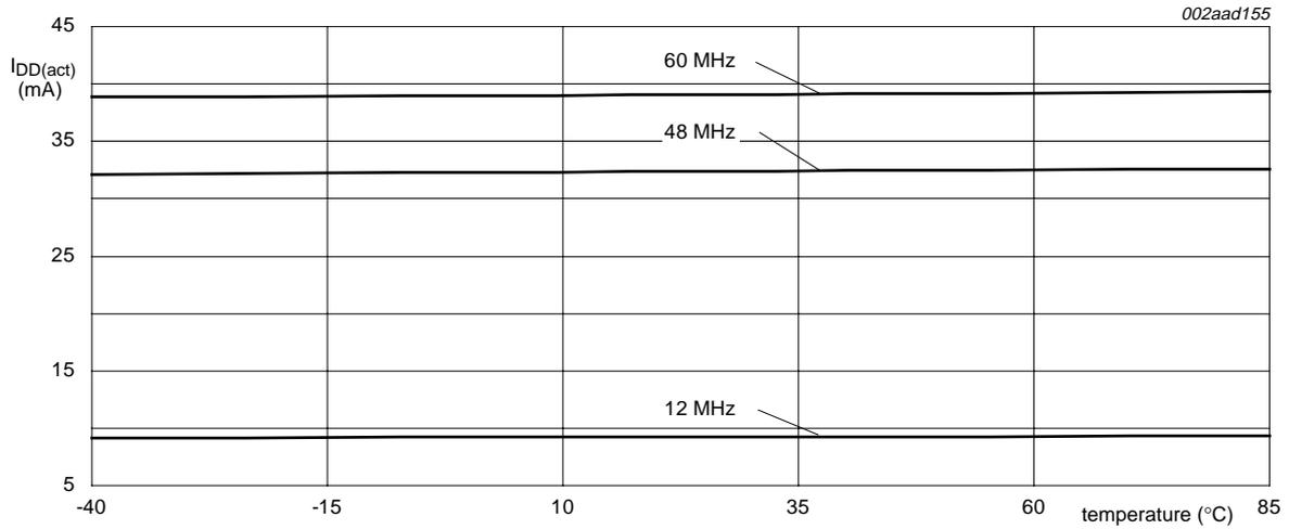
Test conditions: Active mode entered executing code from on-chip flash; PCLK = CCLK<sub>4</sub>; core voltage 1.8 V; all peripherals disabled.
