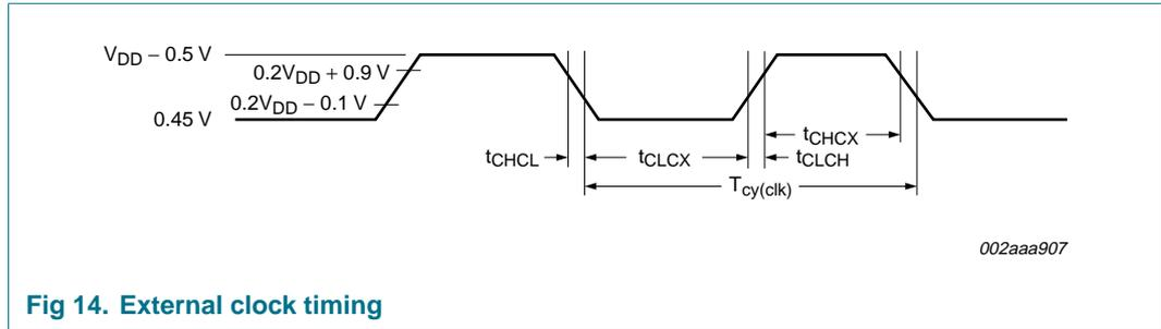
Fig 14. External clock timing
