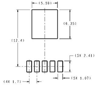
DIMENSIONS ARE IN MILLIMETERS
