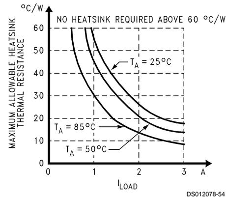
**FIGURE 8. Heatsink Thermal Resistance Requirements for Figure 7**
