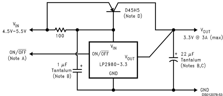
FIGURE 7. 5V to 3.3V @ 3A Converter
