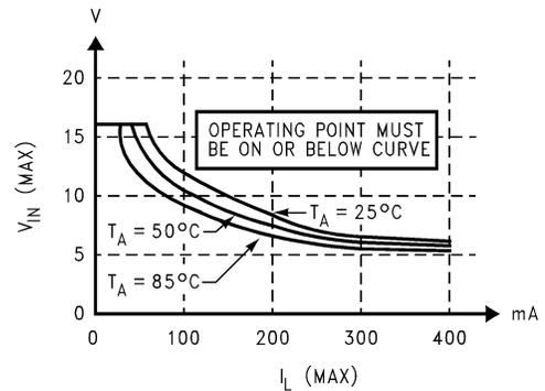
FIGURE 6. Safe Operation Boundary Curves for Figure 5
