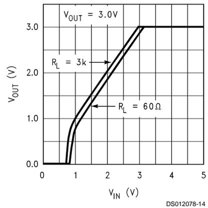
**Typical Performance Characteristics** Unless otherwise specified:  $T_A = 25^\circ\text{C}$ ,  $V_{IN} = V_{O(NOM)} + 1\text{V}$ ,  $C_{OUT} = 2.2\ \mu\text{F}$ , all voltage options, ON/OFF pin tied to  $V_{IN}$ . (Continued)
