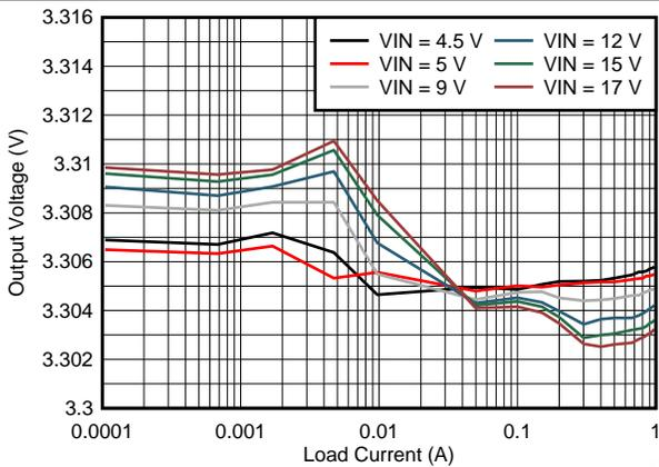
Figure 66. Line and Load Regulation  $V_{OUT} = 3.3\text{ V}$
