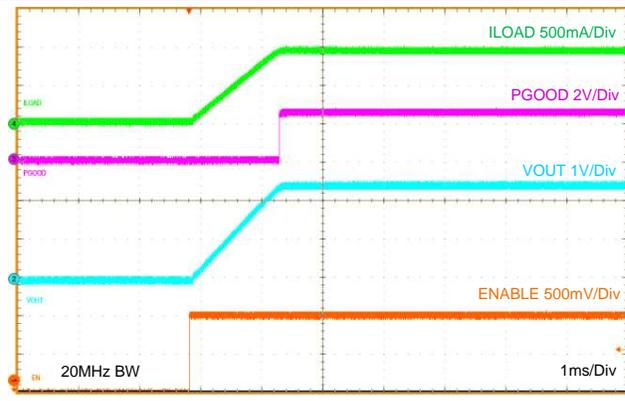
Figure 49. Startup  $V_{OUT} = 2.5\text{ V}$
