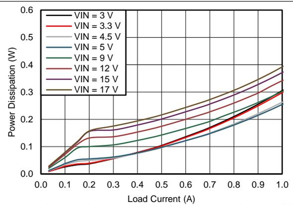
Figure 23. Power Dissipation  $V_{OUT} = 1.2\text{ V}$
