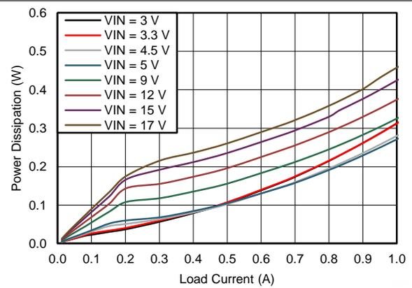
Figure 35. Power Dissipation  $V_{OUT} = 1.8\text{ V}$
