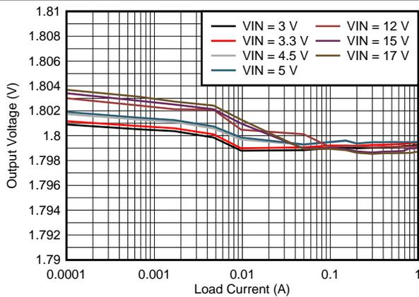
Figure 42. Line and Load Regulation  $V_{OUT} = 1.8\text{ V}$
