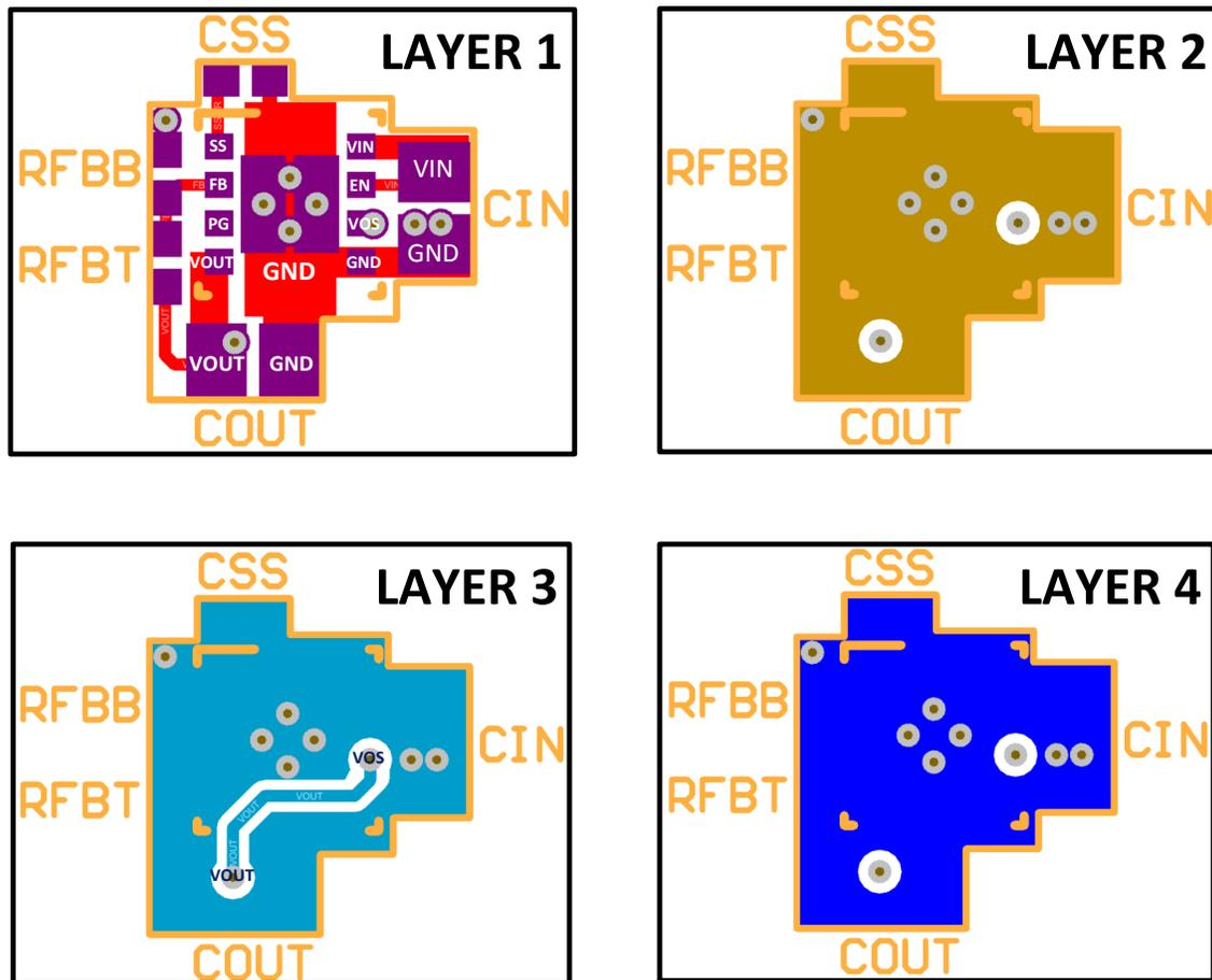
**Figure 82. 35 mm<sup>2</sup> Solution Size (Single Sided)**
