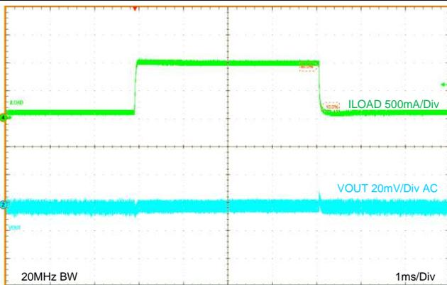
Figure 36. Load Transient  $V_{OUT} = 1.8\text{ V}$
