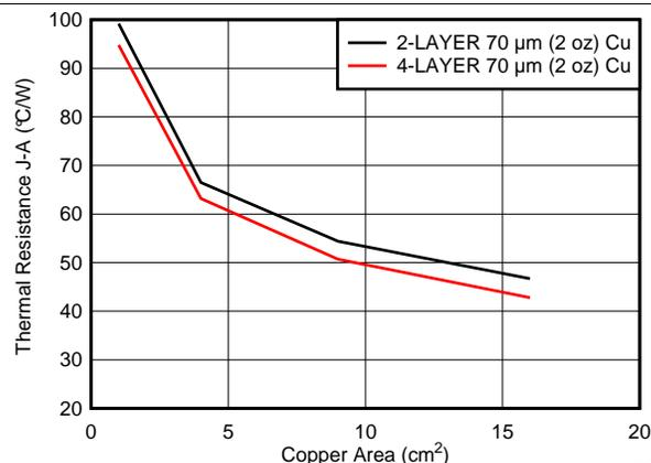
Figure 80. Package Thermal Resistance vs. Board Copper Area
