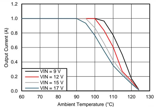
Figure 79. Thermal Derating for  $\theta_{JA} = 47\text{ }^\circ\text{C/W}$ ,  $V_{OUT} = 5.0\text{ V}$
