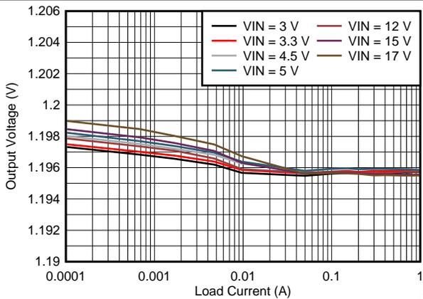
Figure 30. Line and Load Regulation  $V_{OUT} = 1.2\text{ V}$
