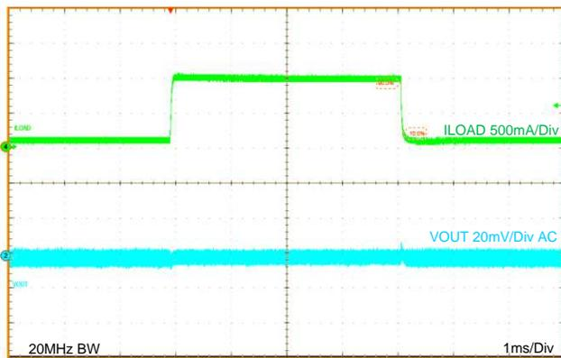
Figure 24. Load Transient  $V_{OUT} = 1.2\text{ V}$
