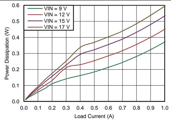
Figure 71. Power Dissipation  $V_{OUT} = 5.0\text{ V}$
