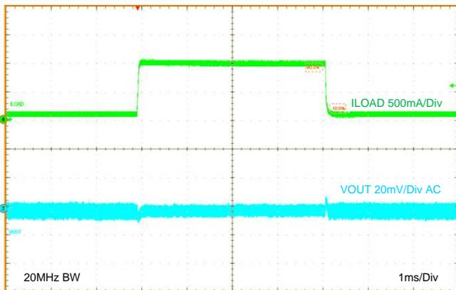
Figure 60. Load Transient  $V_{OUT} = 3.3\text{ V}$
