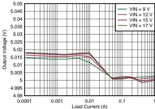
Figure 78. Line and Load Regulation  $V_{OUT} = 5.0\text{ V}$
