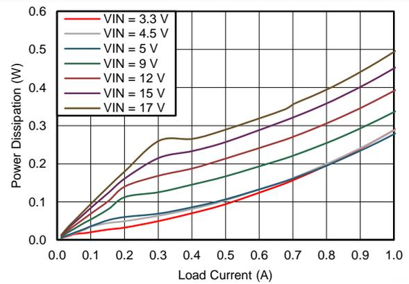
Figure 47. Power Dissipation  $V_{OUT} = 2.5\text{ V}$
