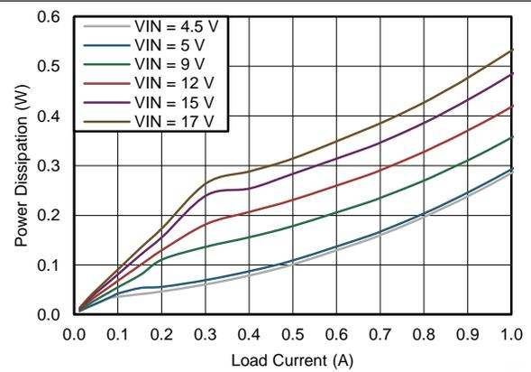
Figure 59. Power Dissipation  $V_{OUT} = 3.3\text{ V}$
