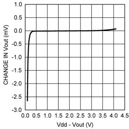
**Figure 7. Change in Vout vs Overhead Voltage**
