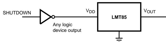
**Figure 14. Simple Shutdown Connection of the LMT85**
