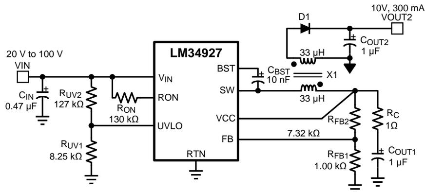
Figure 18. Lowest Part Count Isolated Application Schematic
