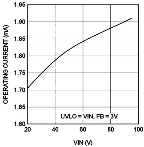
Figure 10.  $I_{IN}$  vs  $V_{IN}$  (Operating, Non Switching)
