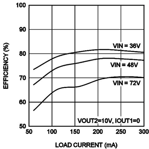
Figure 4. Efficiency at 750 kHz,  $V_{OUT1} = 10\text{ V}$
