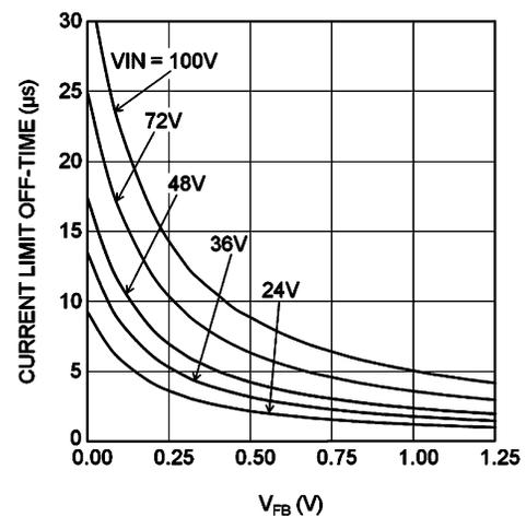
Figure 9.  $T_{OFF} (I_{LIM})$  vs  $V_{FB}$  and  $V_{IN}$
