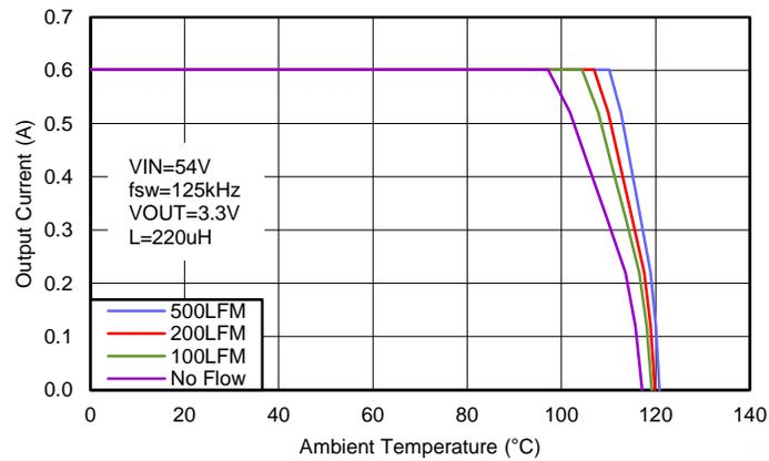
Figure 29. Thermal Derating Curve
