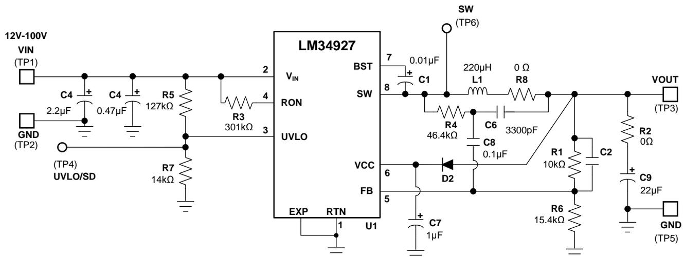
Figure 21. Typical Buck Configuration:
