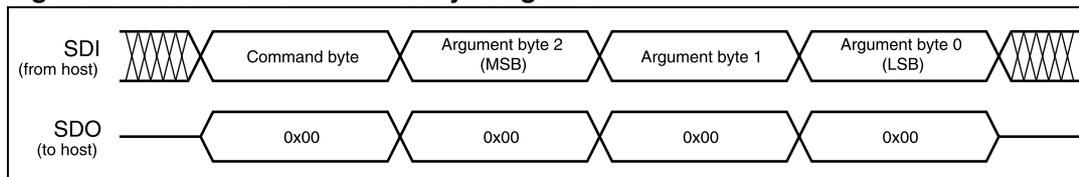
By default, the device returns an all zeroes response for any received byte, the only exceptions are GetParam and GetStatus commands. When one of these commands is received, the following response bytes represent the related register value (see [Figure 16](#)).
