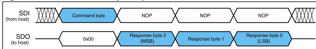
During response transmission, new commands can be sent. If a command requiring a response is sent before the previous response is completed, the response transmission is aborted and the new response is loaded into the output communication buffer (see [Figure 24](#)).
