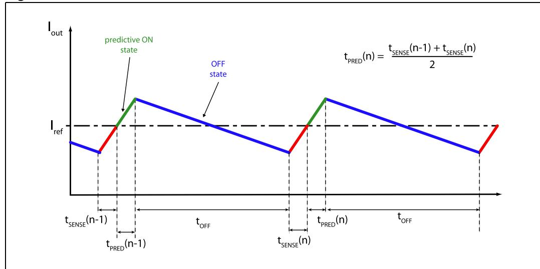
At the end of the predictive ON state the power stage is set in the OFF state for a fixed time, as in a constant  $t_{OFF}$  current control. During the OFF state both slow and fast decay can be performed; the better decay combination is automatically selected by the L6472, as described in [Section 7.2](#).
