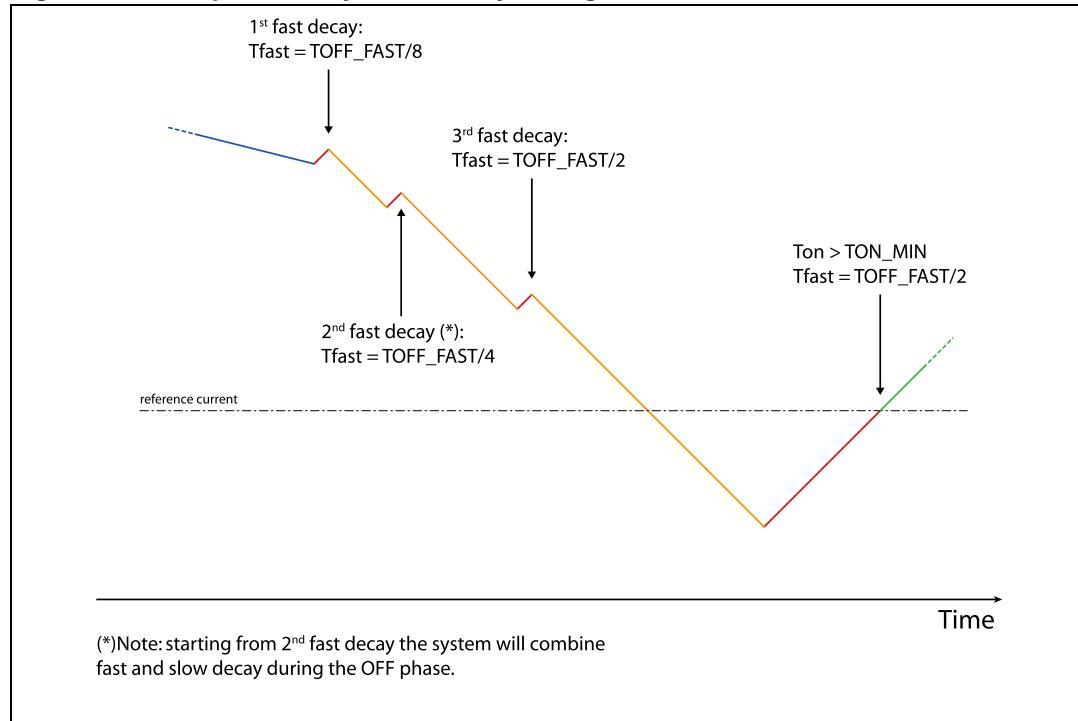
When two or more fast decays are performed with the present target current, the control system adds a fast decay at the end of every OFF time, keeping the OFF state duration constant ( $t_{OFF}$  is split into  $t_{OFF,SLOW}$  and  $t_{OFF,FAST}$ ). When the current threshold is increased by a microstep change (rising step), the system returns to normal decay mode (slow decay only) and the  $t_{FAST}$  value is halved.
