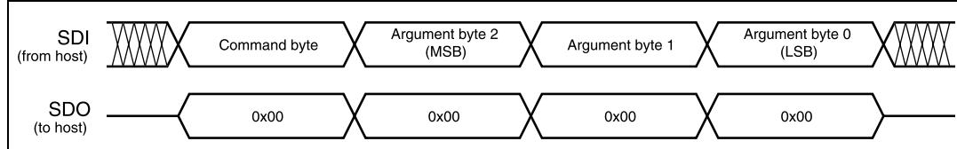
By default the device returns an all zeroes response for any received byte, the only exceptions are GetParam and GetStatus commands. When one of these commands is received the following response bytes represents the related register value (see [Figure 23](#)).
