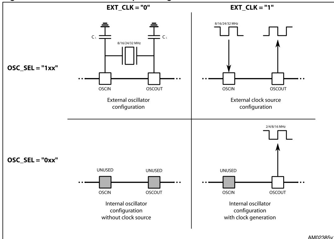
**Note:***When OSCIN is UNUSED, it should be left floating.**When OSCOUT is UNUSED it should be left floating.*
