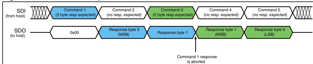
When a byte that does not correspond to a command is sent to the IC, it is ignored and the `WRONG_CMD` flag in the `STATUS` register is raised (see [Section 9.1.19](#)).
