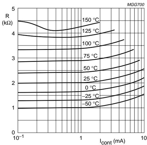
To keep the temperature error low, an operating current of I<sub>cont</sub> = 1 mA is recommended for temperatures above 100 °C.
