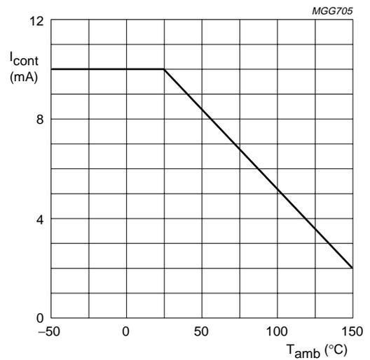
Fig.5 Maximum operating current for safe operation.
