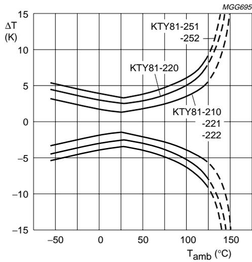
Fig.2 Maximum expected temperature error (ΔT).
