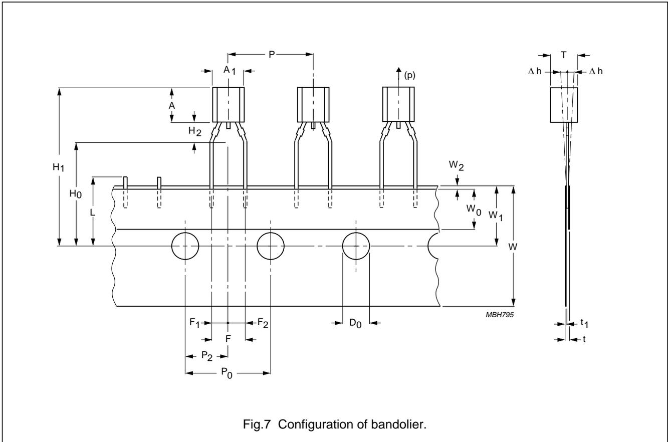
Fig.7 Configuration of bandolier.
