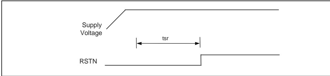
**Figure 18. Reset Timing**
