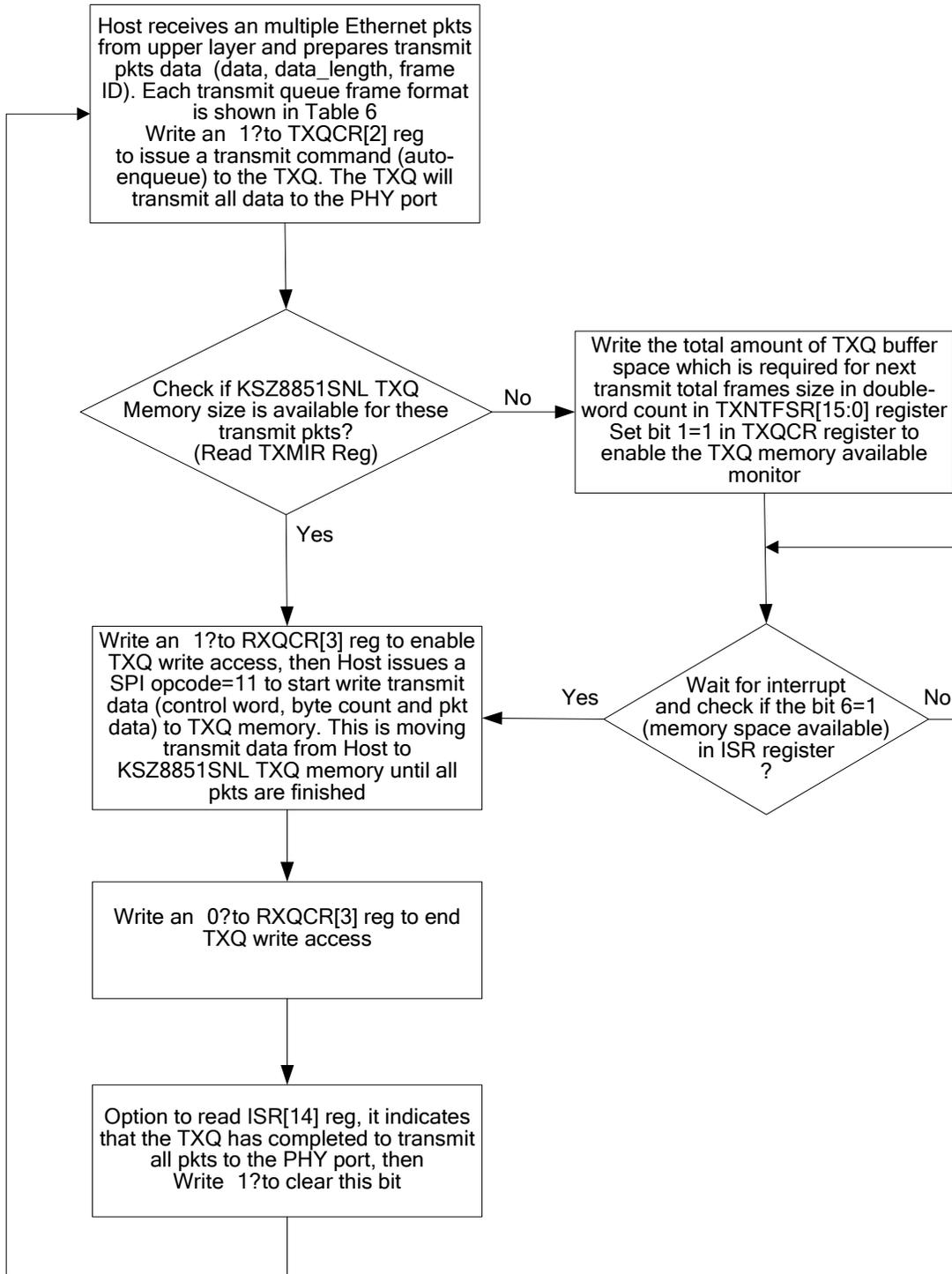
Figure 12. Host TX Multiple Frames in Auto- Enqueue Flow Diagram
