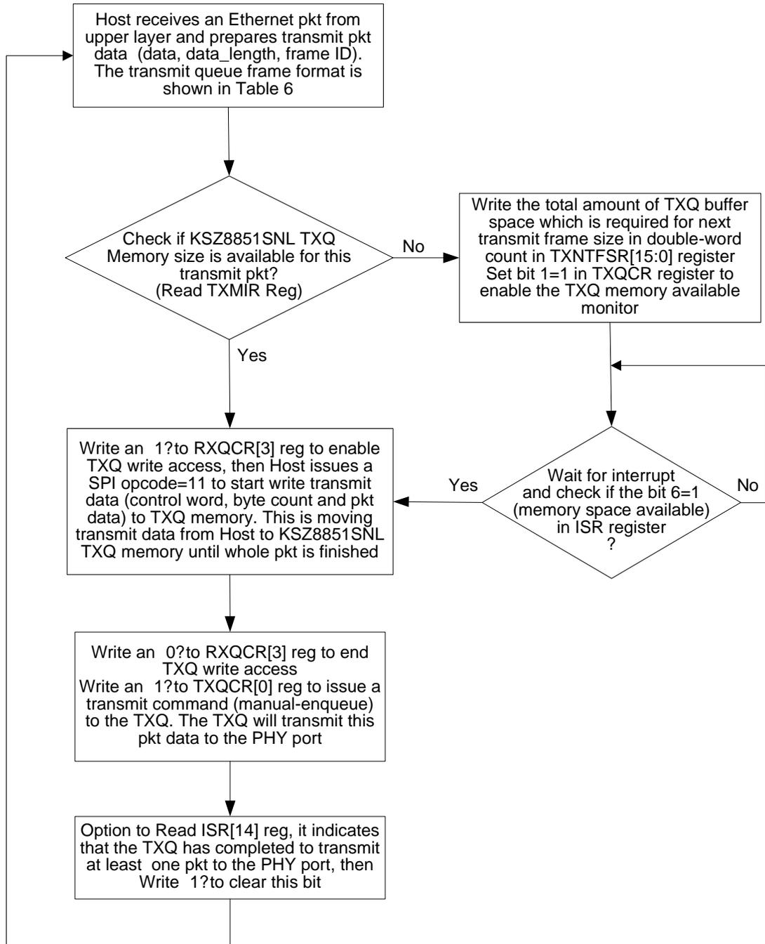
Figure 11. Host TX Single Frame in Manual Enqueue Flow Diagram
