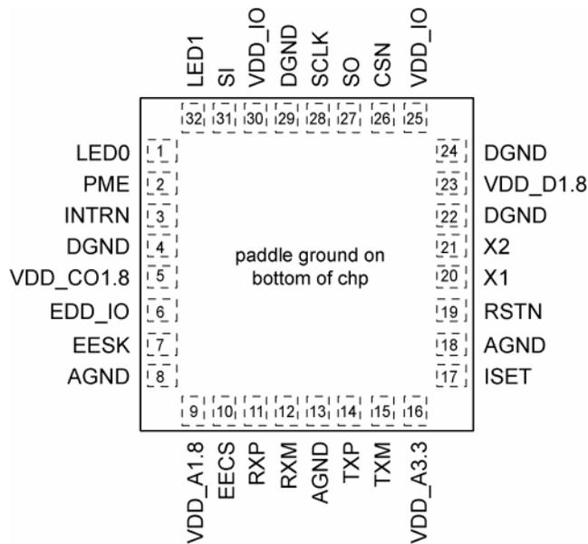
Figure 2. 32-Pin (5mm x 5mm) MLF<sup>®</sup>
