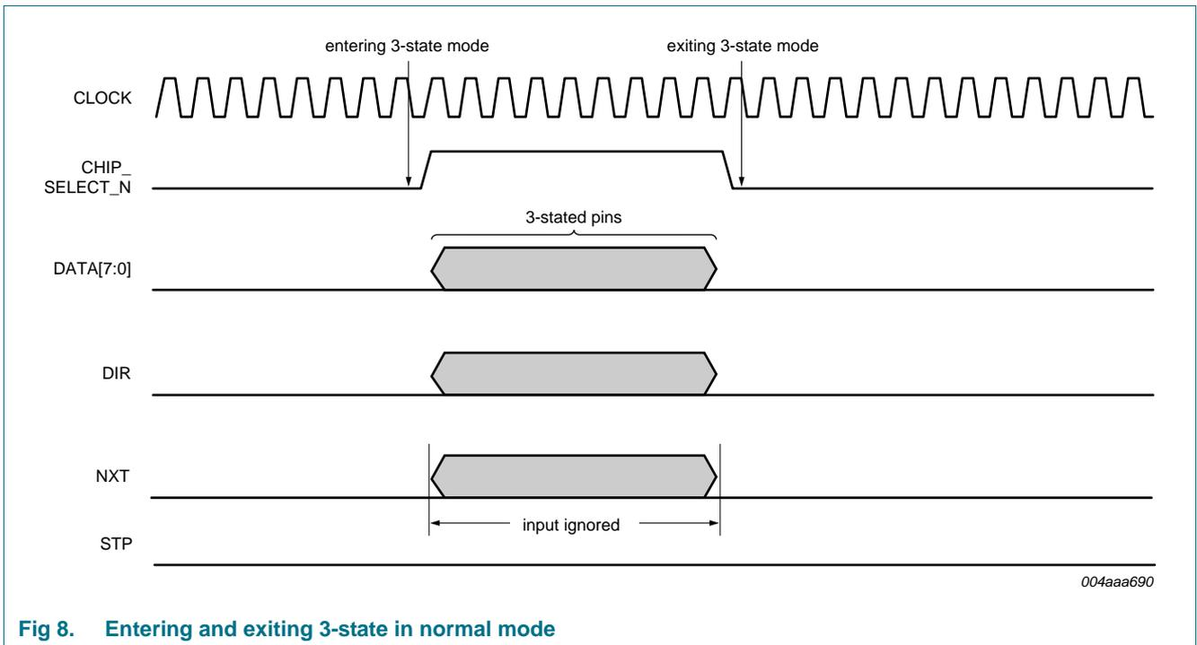
**Fig 8. Entering and exiting 3-state in normal mode**
