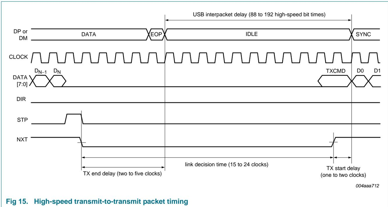
**Fig 15. High-speed transmit-to-transmit packet timing**
