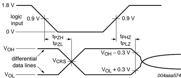
Fig 31. Timing of TX\_ENABLE to DP and DM
