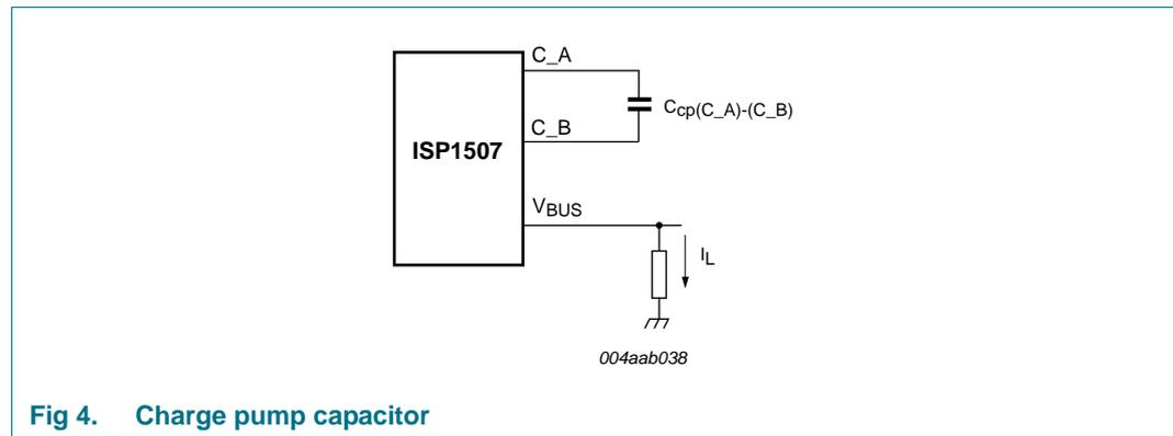
**Fig 4. Charge pump capacitor**
