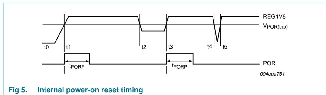
Fig 5. Internal power-on reset timing
