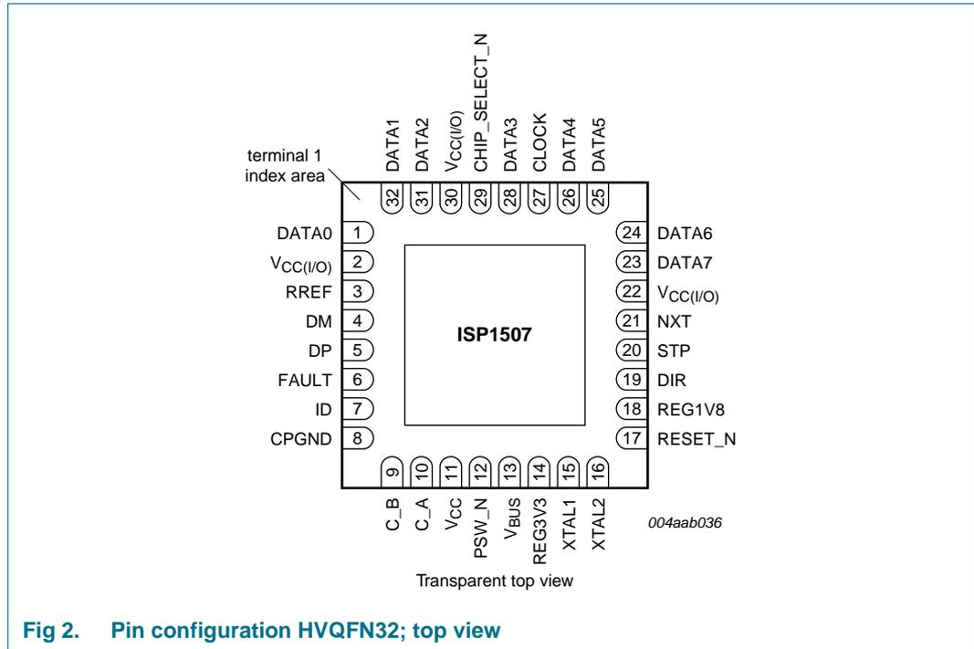
Fig 2. Pin configuration HVQFN32; top view
