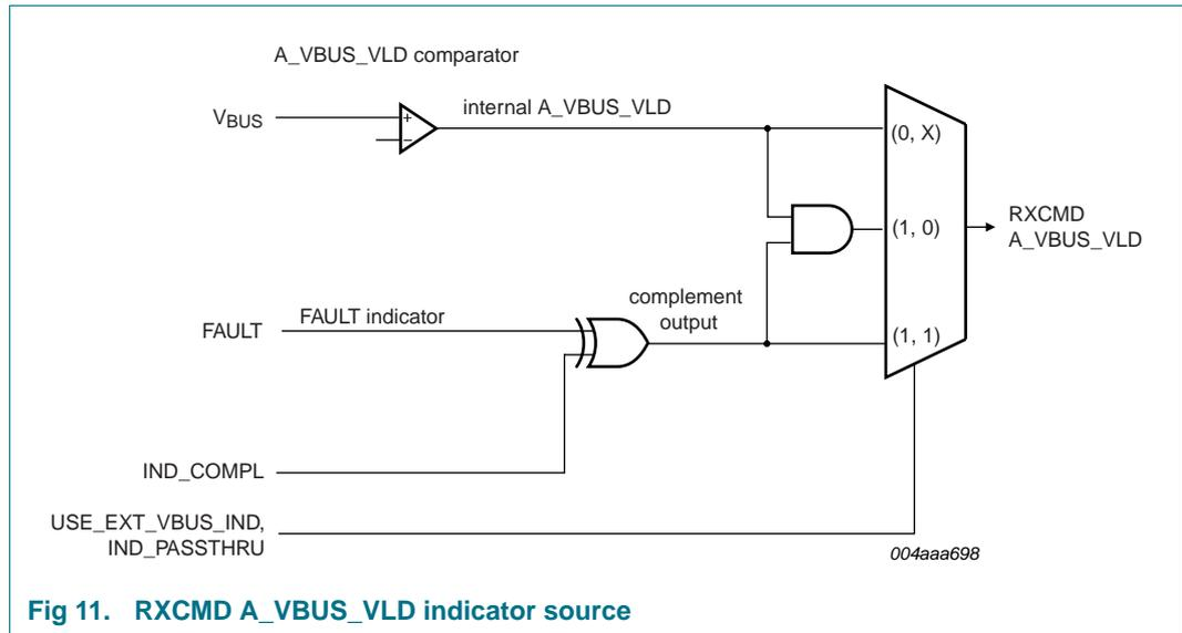
**Fig 11. RXCMD A\_VBUS\_VLD indicator source**
