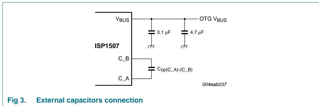
Fig 3. External capacitors connection
