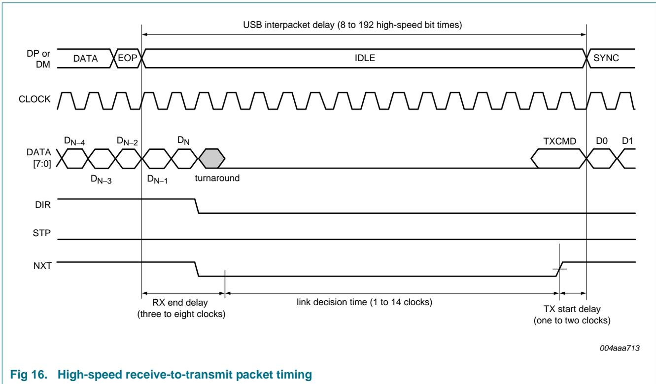
**Fig 16. High-speed receive-to-transmit packet timing**
