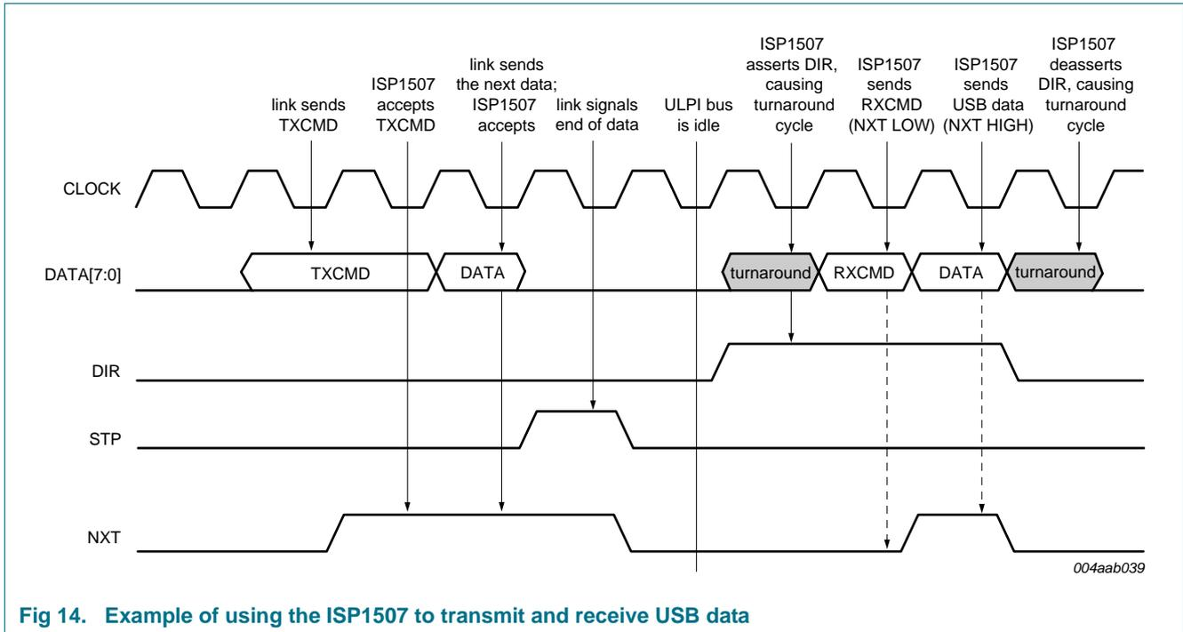
**Fig 14. Example of using the ISP1507 to transmit and receive USB data**
