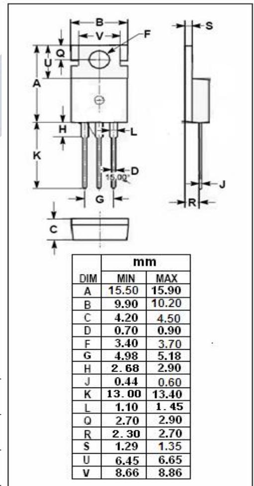
**isc N-Channel MOSFET Transistor IPP200N25N3, IIPP200N25N3**
