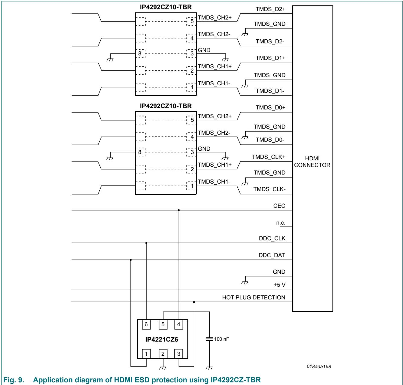
Fig. 9. Application diagram of HDMI ESD protection using IP4292CZ-TBR
