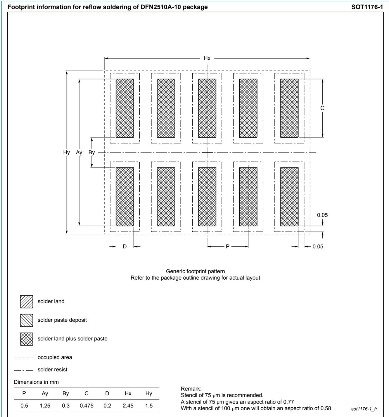
Fig. 11. Reflow soldering footprint for DFN2510A-10 (SOT1176-1)
