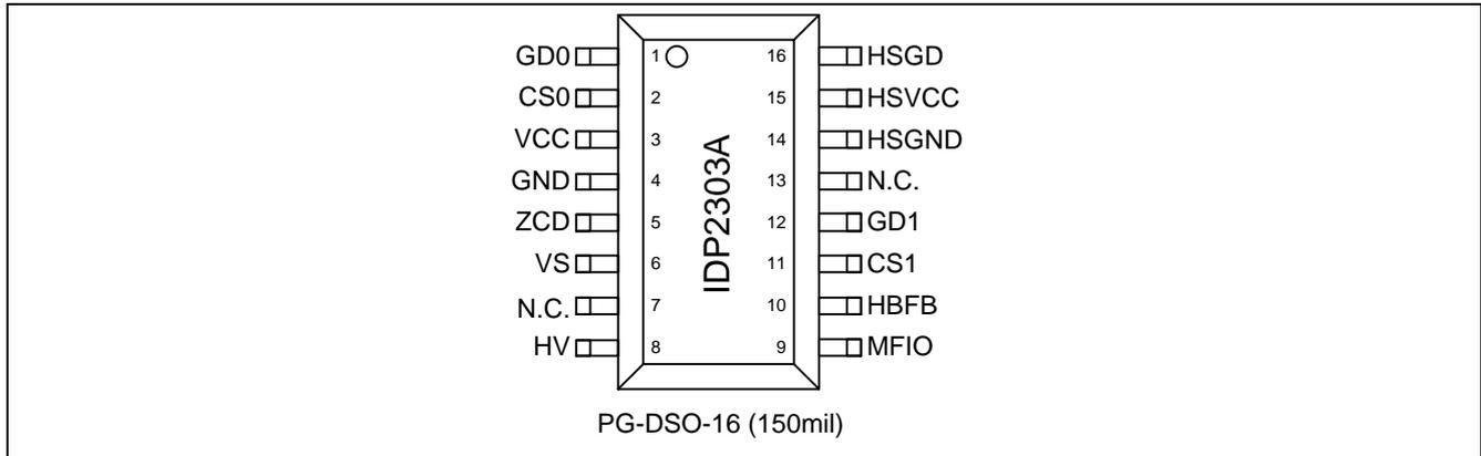
**Figure 2 Pin Configuration**
