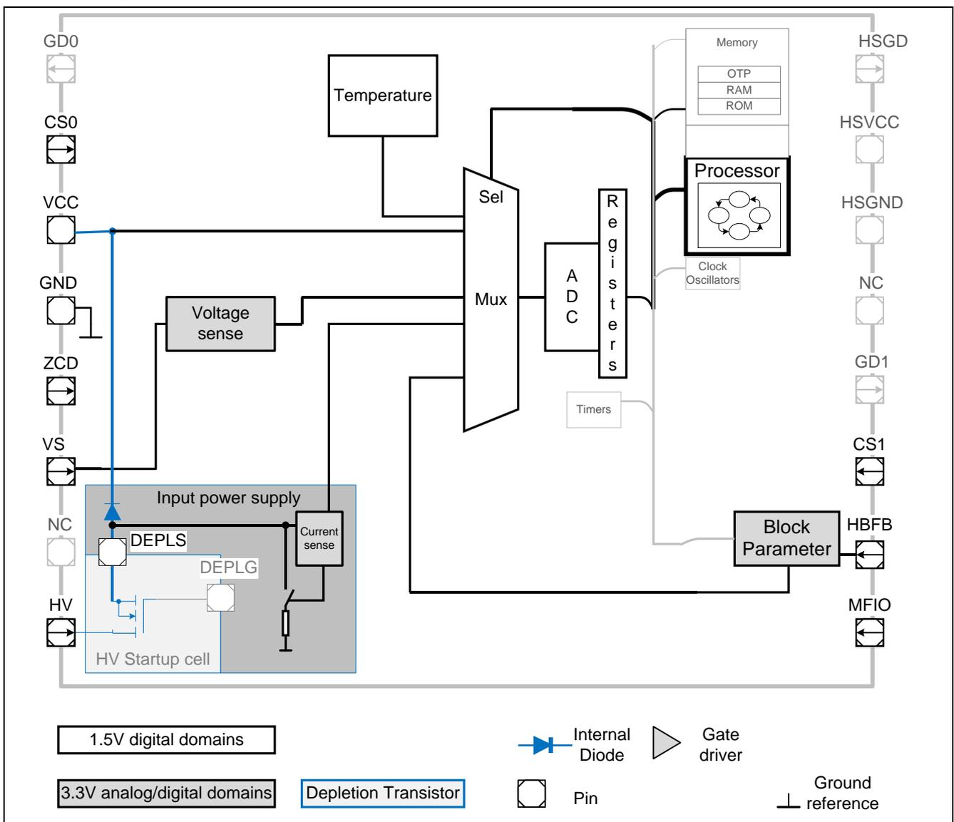
Figure 6 Voltage and current sensing multiplexing to ADC
