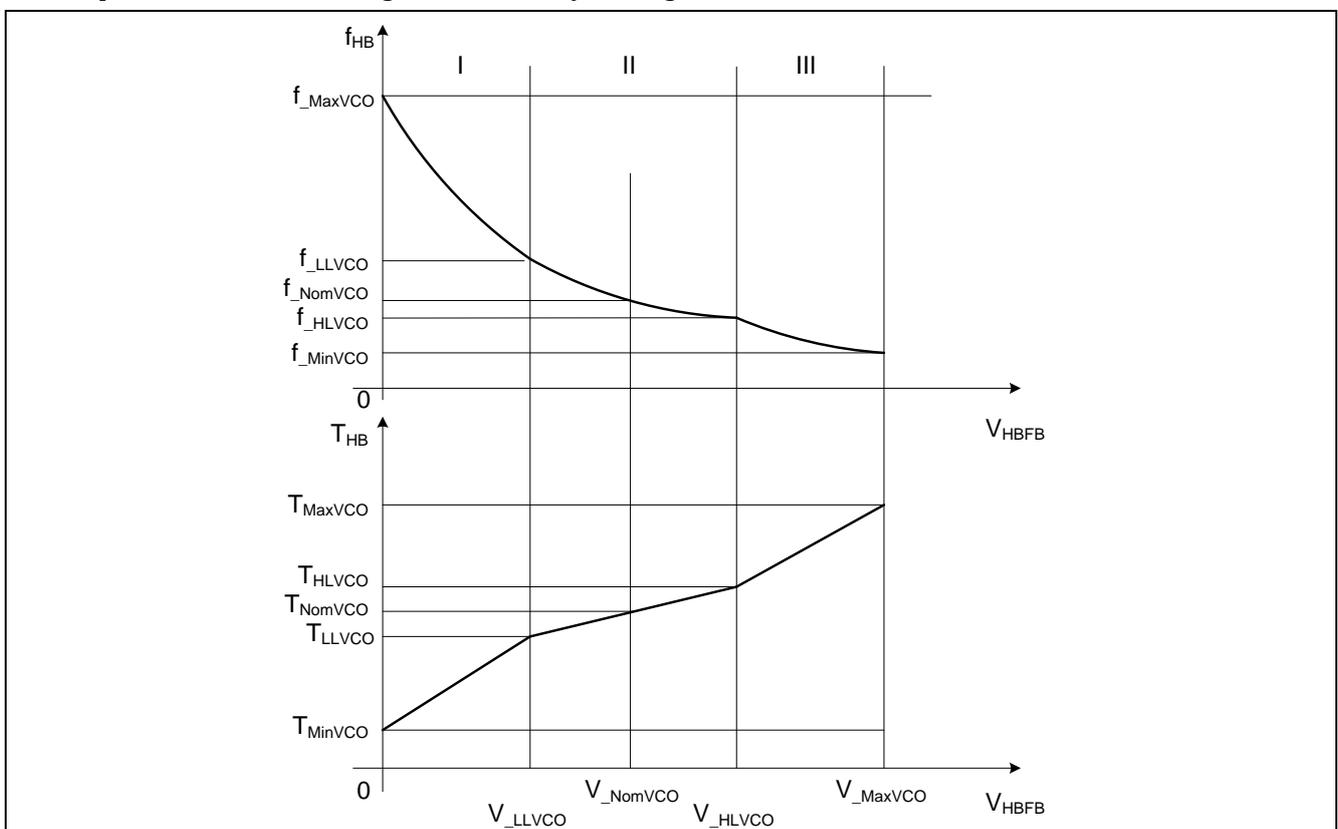
Figure 13 Frequency vs. Feedback Voltage of the VCO
