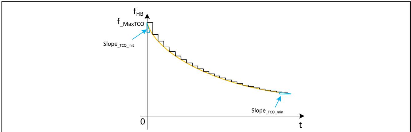
Figure 12 Frequency vs. Time of the TCO
