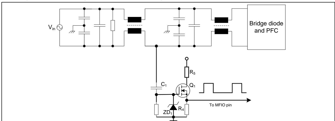
Figure 9 Circuit with AC detection with EMI filter
