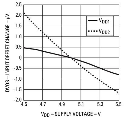
Figure 6. Input offset change vs. supply voltage.
