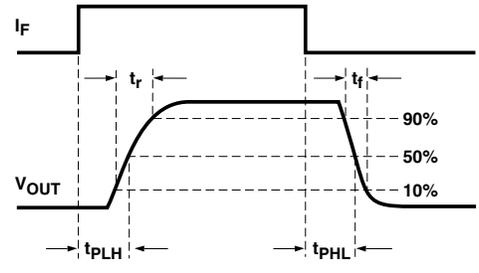
Figure 17. Propagation Delay Test Circuit and Waveforms.
