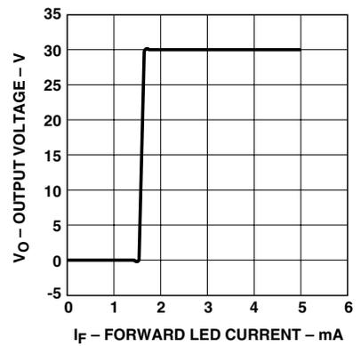
Figure 15. Transfer Characteristics.
