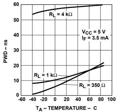
Figure 13. Typical pulse width distortion vs. temperature.
