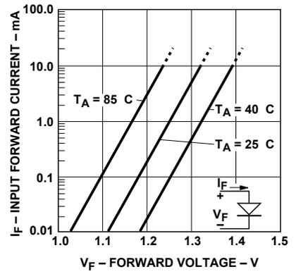
Figure 6. Typical diode input forward current characteristic.
