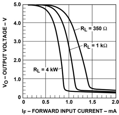
Figure 7. Typical output voltage vs. forward input current.
