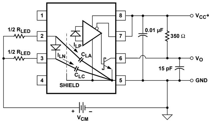
Figure 21. AC equivalent circuit for HCPL-261X.
