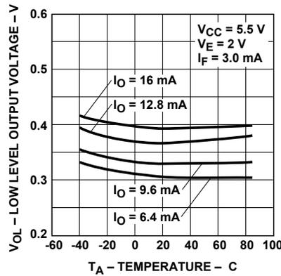
Figure 8. Typical low level output voltage vs. temperature.
