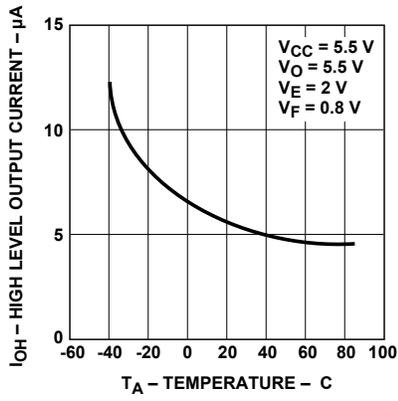
Figure 4. Typical high level output current vs. temperature.
