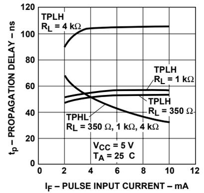
Figure 12. Typical propagation delay vs. pulse input current.
