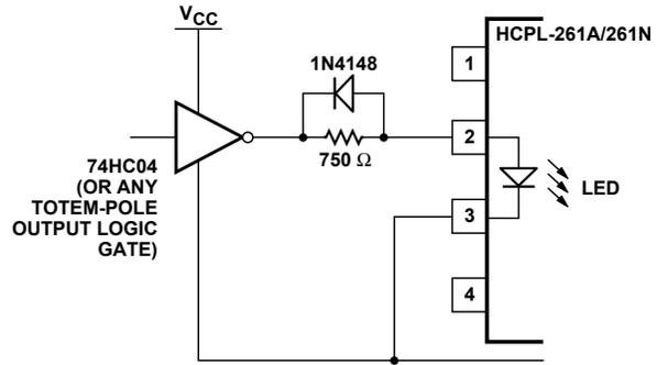
Figure 24. CMOS gate drive circuit for HCPL-261A/-261N families.
