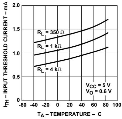
Figure 10. Typical input threshold current vs. temperature.
