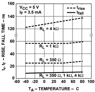
Figure 14. Typical rise and fall time vs. temperature.
