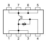
These devices are MOS type. Users should follow proper ESD handling procedures. Operating condition of turn-off dv/dt should be lower than 400 V/ $\mu s$ .
