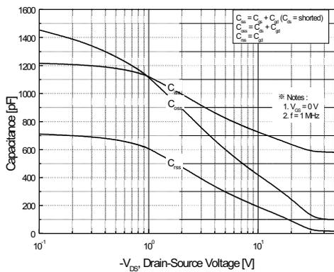
Figure 5. Capacitance Characteristics
