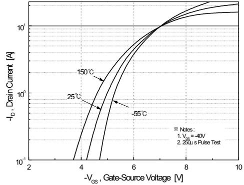
Figure 2. Transfer Characteristics
