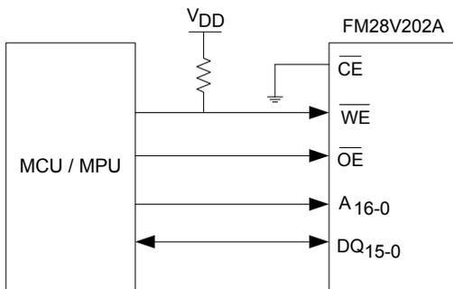
For applications that require the lowest power consumption, the  $\overline{CE}$  signal should be active (LOW) only during memory accesses. The FM28V202A draws supply current while  $\overline{CE}$  is LOW, even if addresses and control signals are static. While  $\overline{CE}$  is HIGH, the device draws no more than the maximum standby current,  $I_{SB}$ .
