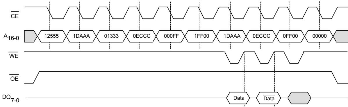
Figure 5. Sequence to Read Write-Protect Settings [1]
