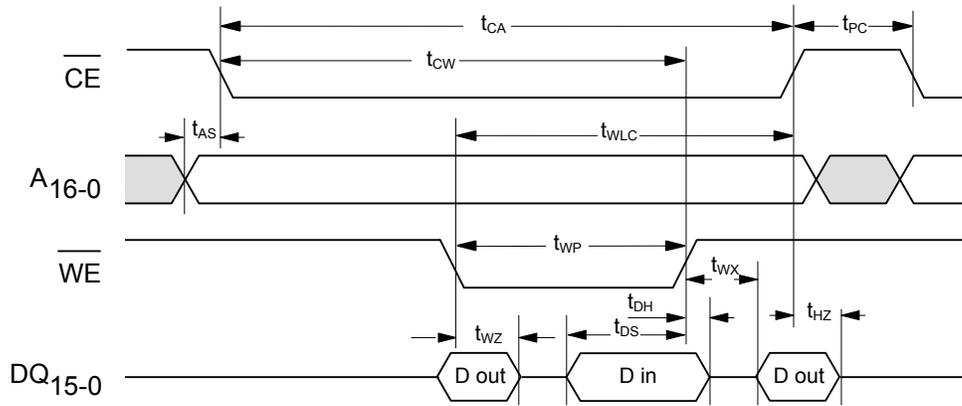
**Figure 12. Write Cycle Timing 2 ( $\overline{CE}$  Controlled)**
