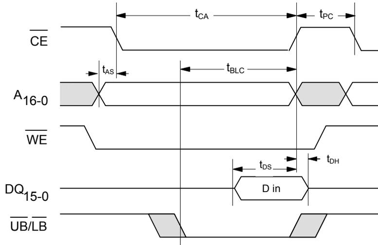
**Figure 13. Write Cycle Timing 3 ( $\overline{CE}$  LOW) [9]**
