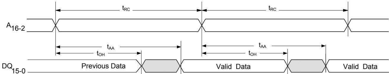
Figure 9. Read Cycle Timing 2 ( $\overline{CE}$  Controlled)
