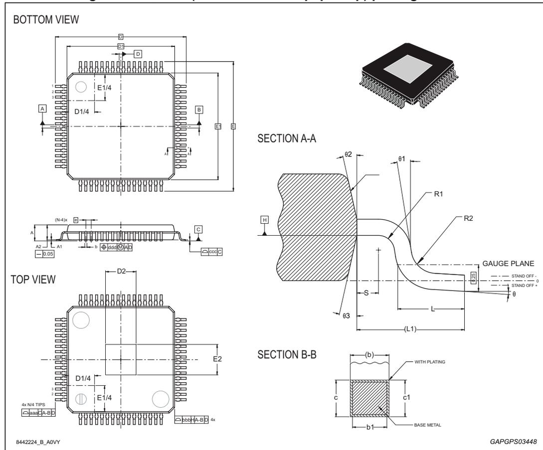
Table 3. LQFP64 (10x10x1.4 mm exp. pad up) package mechanical data
