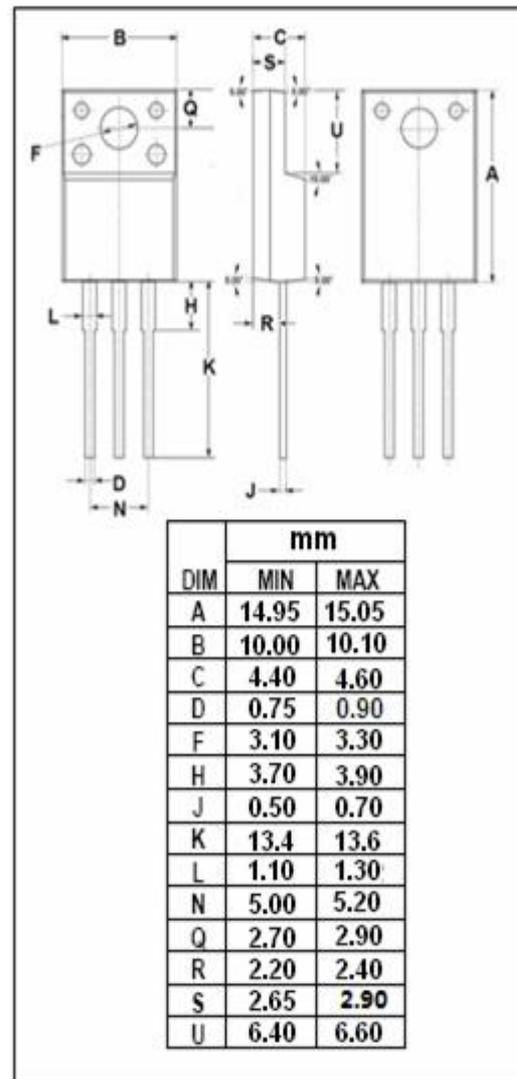
**isc N-Channel MOSFET Transistor****FCPF099N65S3****ELECTRICAL CHARACTERISTICS** $T_c=25^{\circ}\text{C}$  unless otherwise specified
