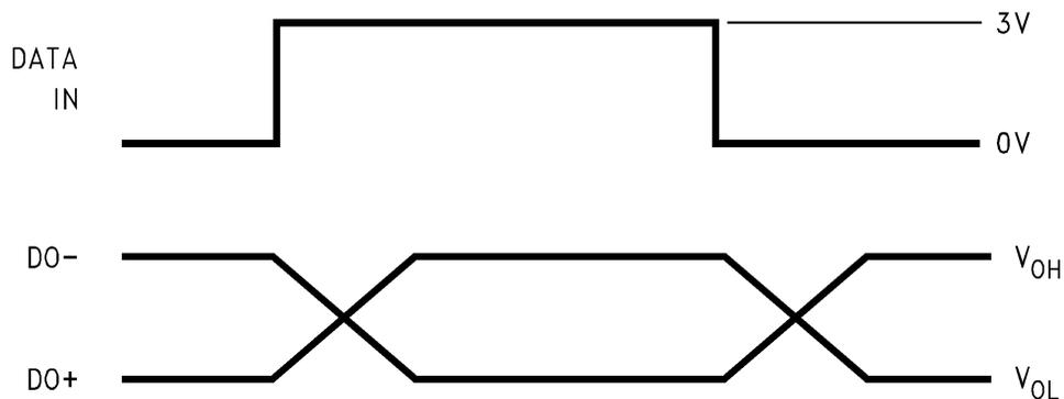
Figure 8. Typical Driver Output Waveforms
