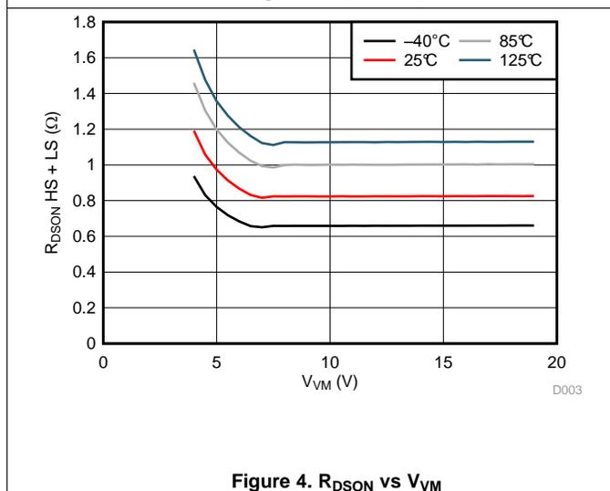
Figure 4. R<sub>DS(on)</sub> vs V<sub>VM</sub>
