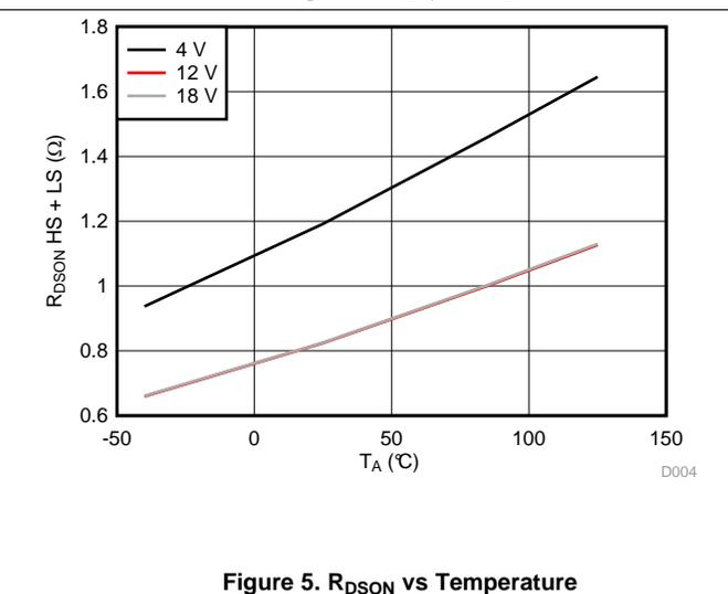
Figure 5. R<sub>DS(on)</sub> vs Temperature
