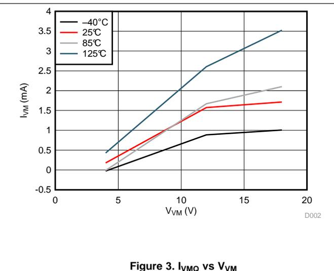
Figure 3. I<sub>VMQ</sub> vs V<sub>VM</sub>
