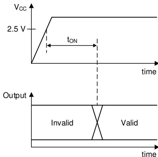
Figure 10.  $t_{ON}$  Definition
