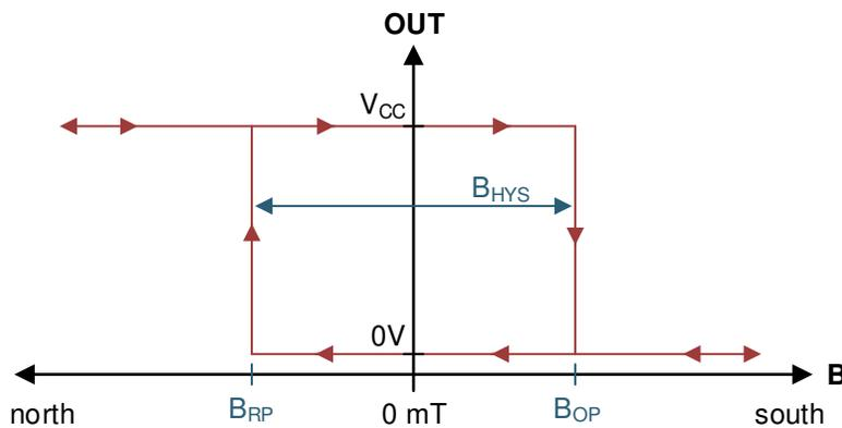
**Figure 8. Device Functionality**
