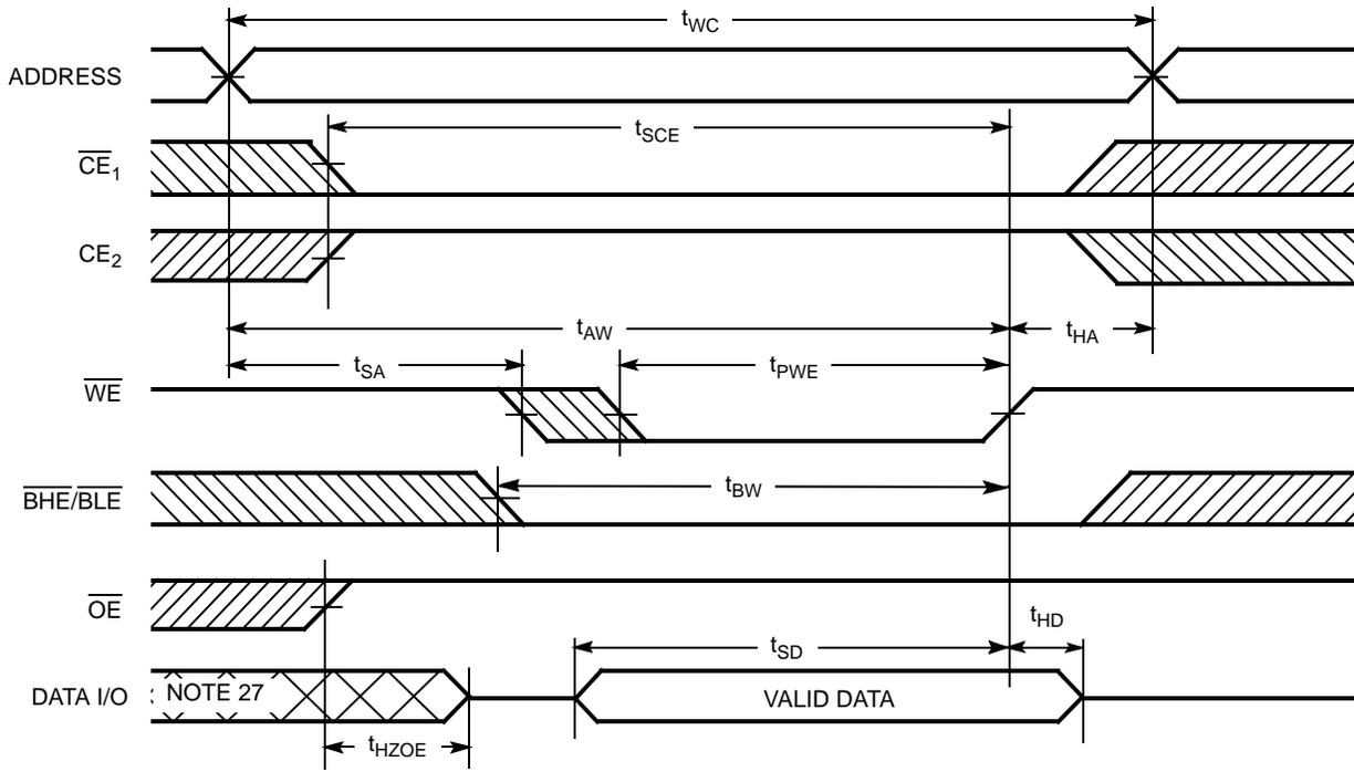
Figure 7. Write Cycle No. 2 ( $\overline{CE}_1$  or  $CE_2$  Controlled)<sup>[24, 25, 26]</sup>
