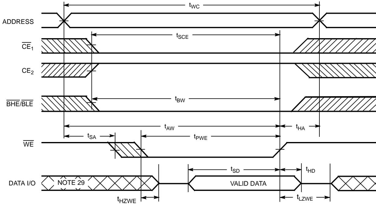
Figure 9. Write Cycle No. 4 ( $\overline{BHE}/\overline{BLE}$  Controlled,  $\overline{OE}$  Low)<sup>[28]</sup>
