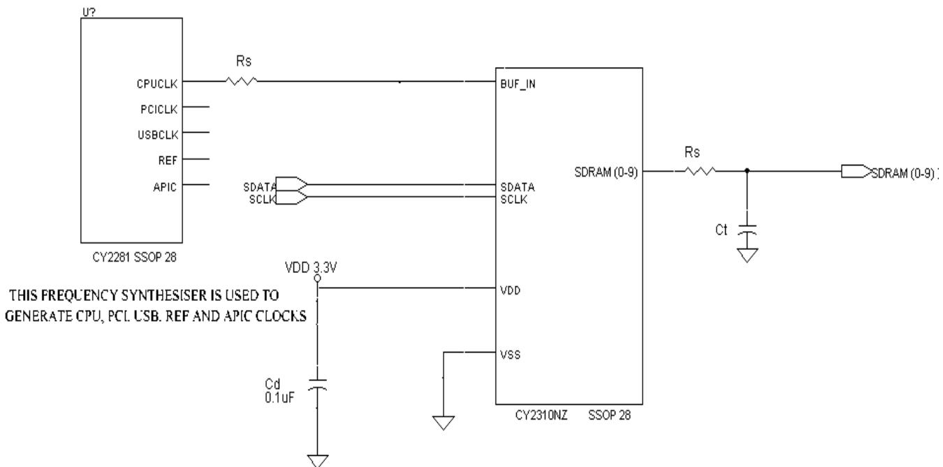
$C_d$  = DECOUPLING CAPACITOR
