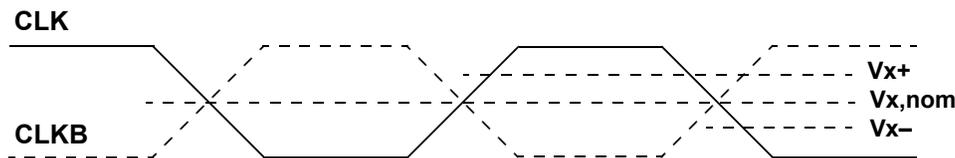
**Figure 6. Crossing-point Voltage**
