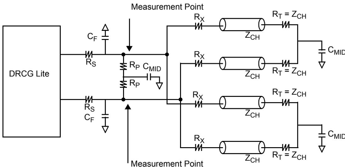
**Figure 4. Output Driving Two Channels**
