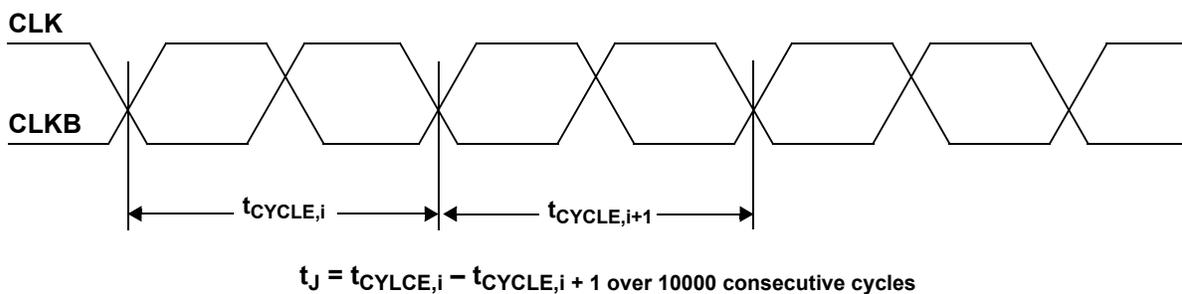
**Figure 9. Cycle-to-cycle Jitter**
