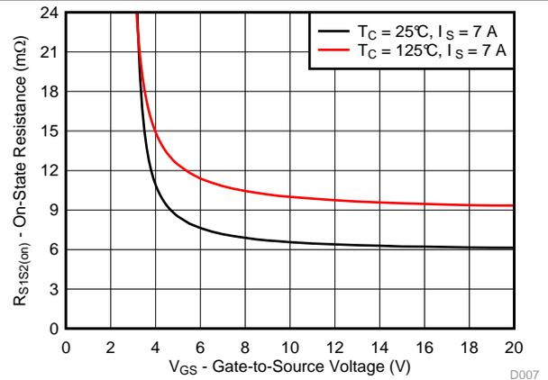
Figure 7. On-State Source-to-Source Resistance vs Gate-to-Source Voltage
