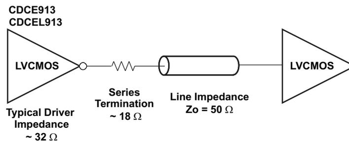
Figure 2. Test Load for 50-Ω Board Environment
