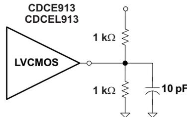
Figure 1. Test Load
