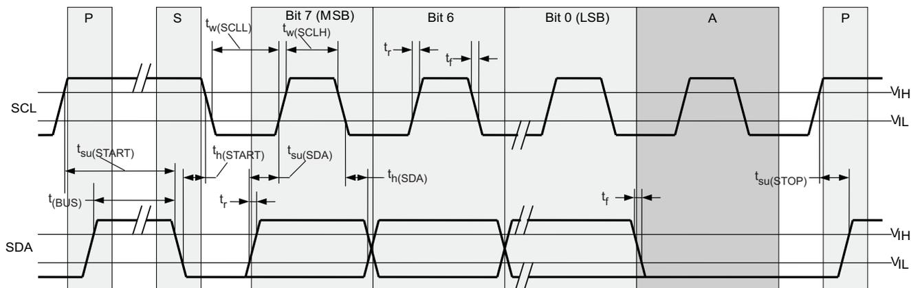
Figure 12. Timing Diagram for SDA/SCL Serial Control Interface
