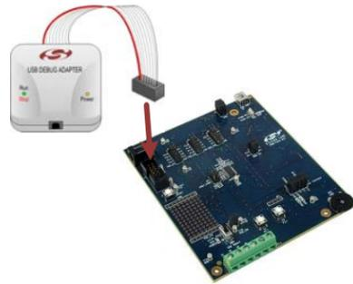
**2** Connect the USB Debug Adapter to the PC using the standard USB cable.
