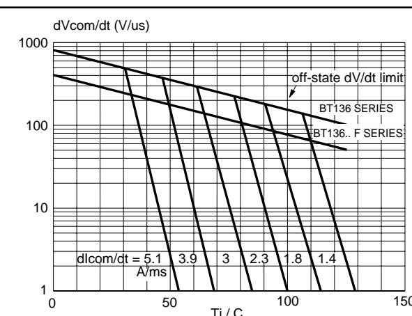
Fig. 12. Typical commutation  $dV/dt$  versus junction temperature, parameter commutation  $dl_{T/dt}$ . The triac should commutate when the  $dV/dt$  is below the value on the appropriate curve for pre-commutation  $dl_{T/dt}$ .
