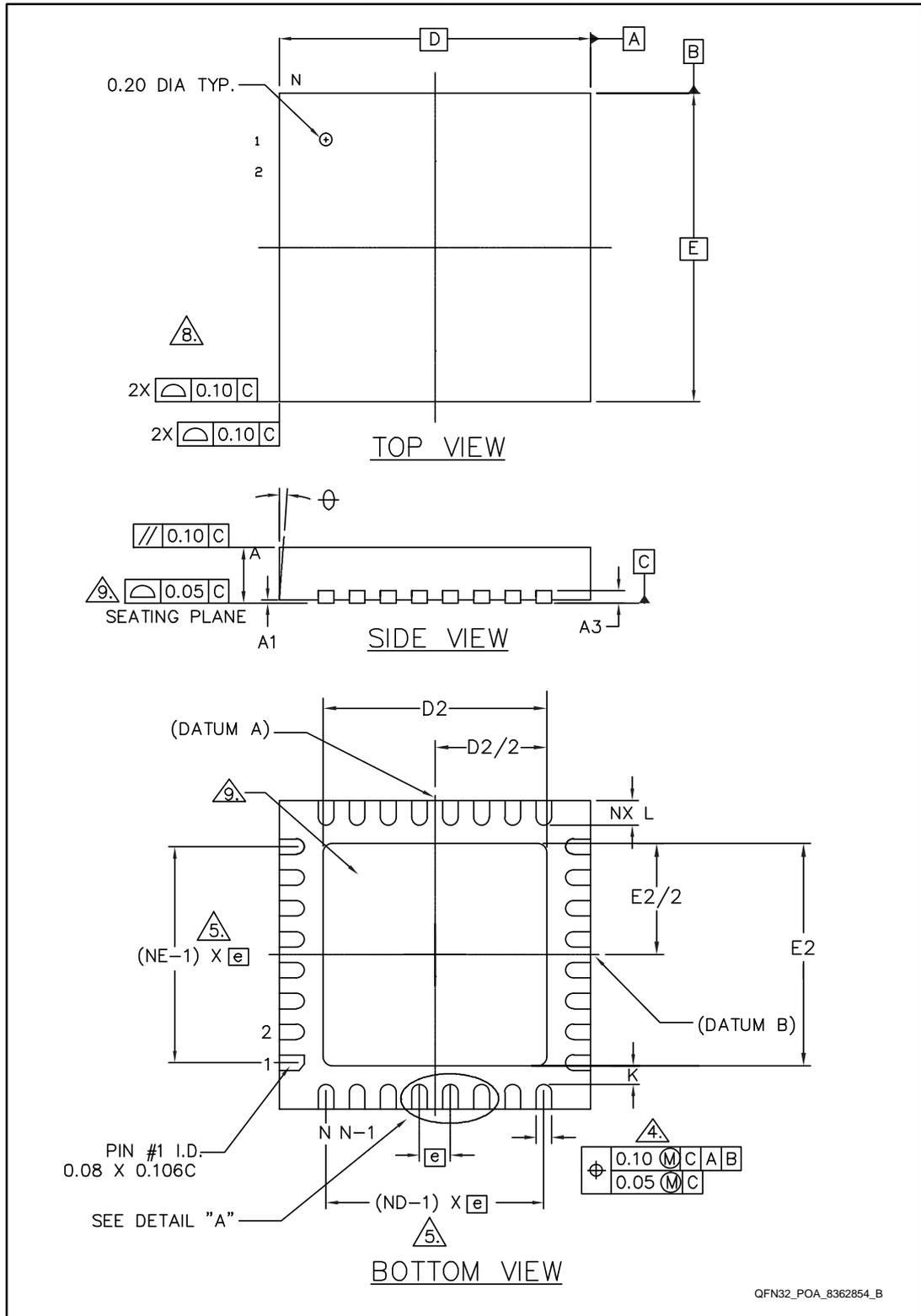
Table 213: QFN32 (5 x 5 x 1 pitch 0.5 mm) mechanical data
