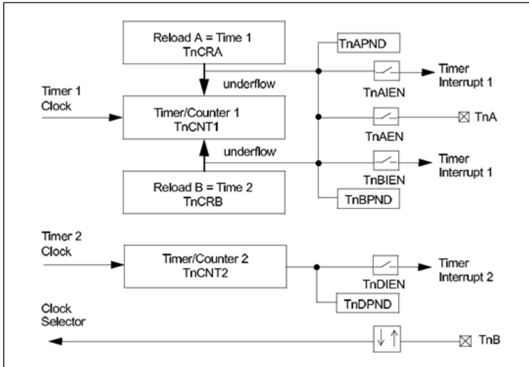
In this mode, the timer toggles the TnA output upon underflow which is connected to PWMx pin of the BlueNRG1. This generates a clock signal on TnA with the width and duty cycle controlled by the values stored in the TnCRB and TnCRA registers.
