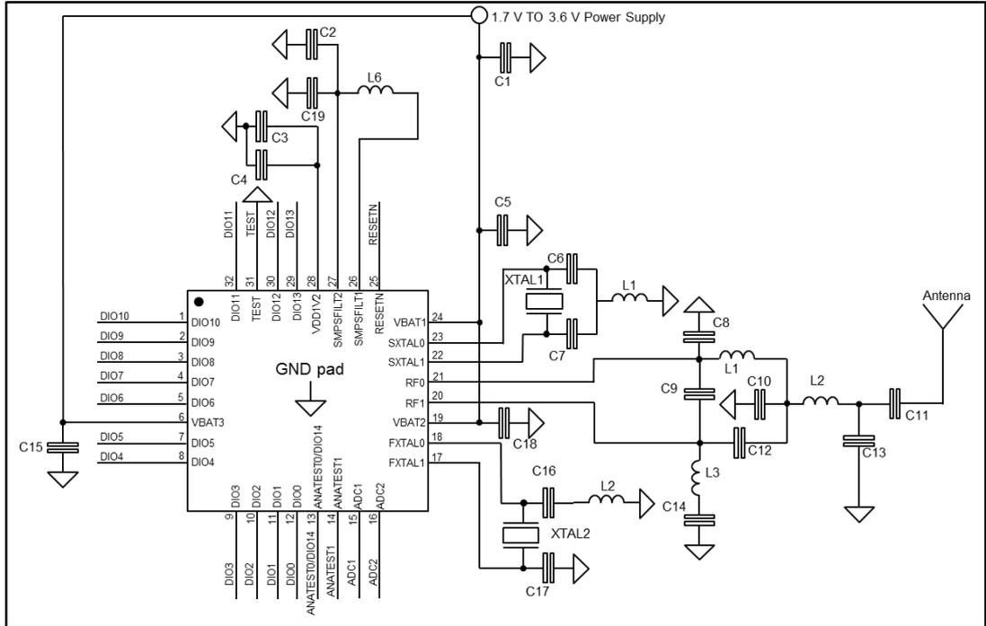
**Figure 21: Application circuit: non-active DC-DC converter QFN32 package**
