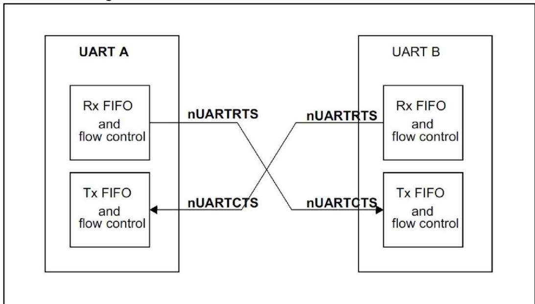
When the RTS flow control is enabled, the UART\_RTS signal is asserted until the receive FIFO is filled up to the programmed watermark level. When the CTS flow control is enabled, the transmitter can only transmit data when the UART\_CTS signal is asserted.
