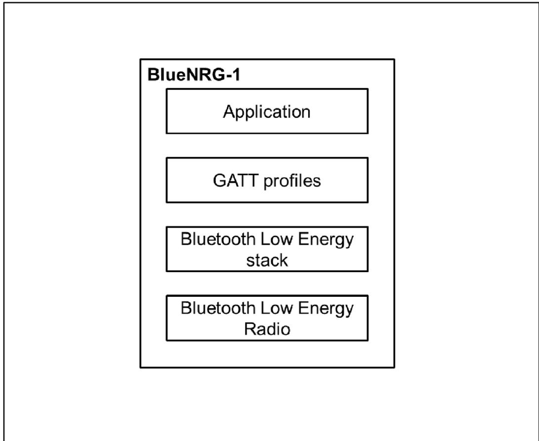
The BlueNRG-1 can be configured for operating as a network coprocessor. In this case a dedicated firmware is provided for supporting the interface with an external application
