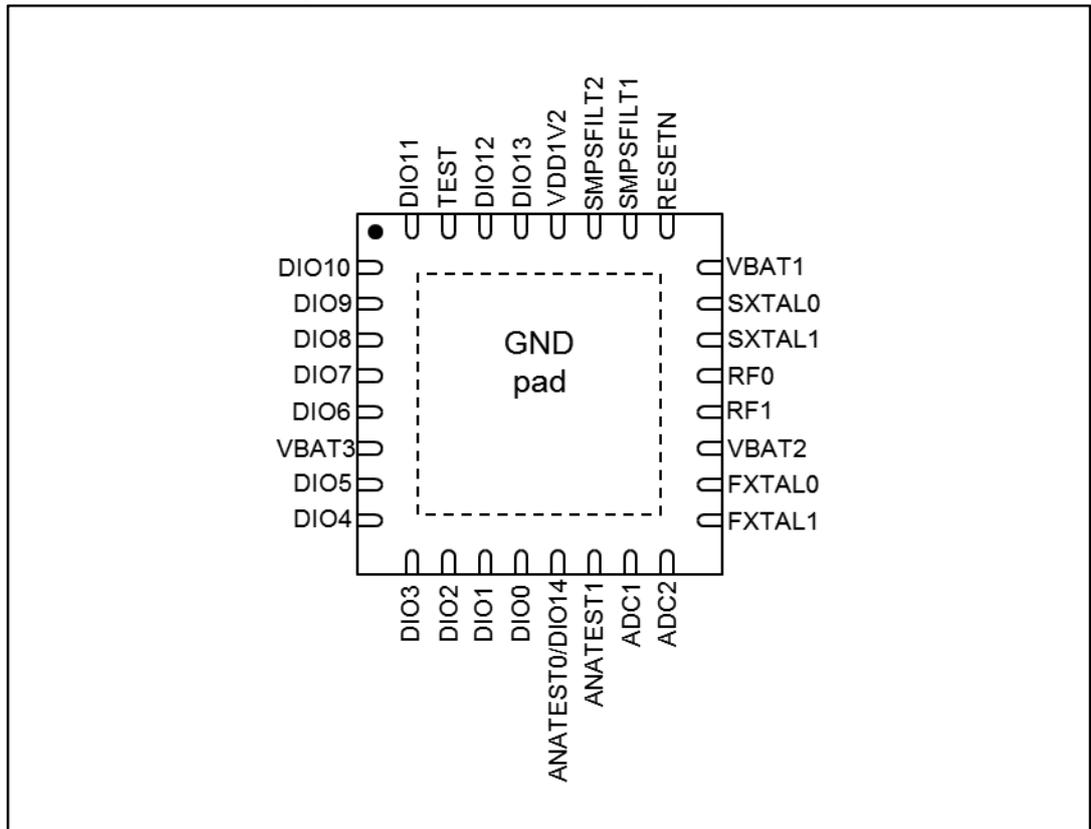
Figure 18: BlueNRG-1 ball out top view (WCSP34)
