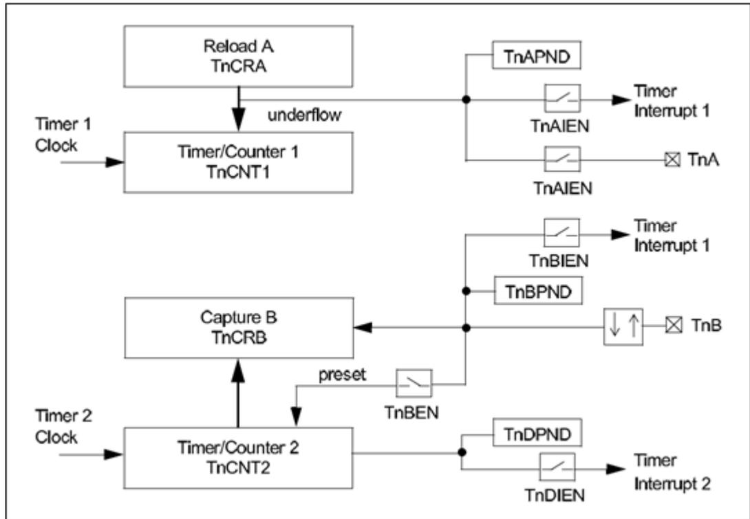
This mode is a combination of mode 3 and mode 2, and makes it possible to operate Timer/Counter 2 as a single input-capture timer while Timer/Counter 1 can be used as a system timer as described above.
