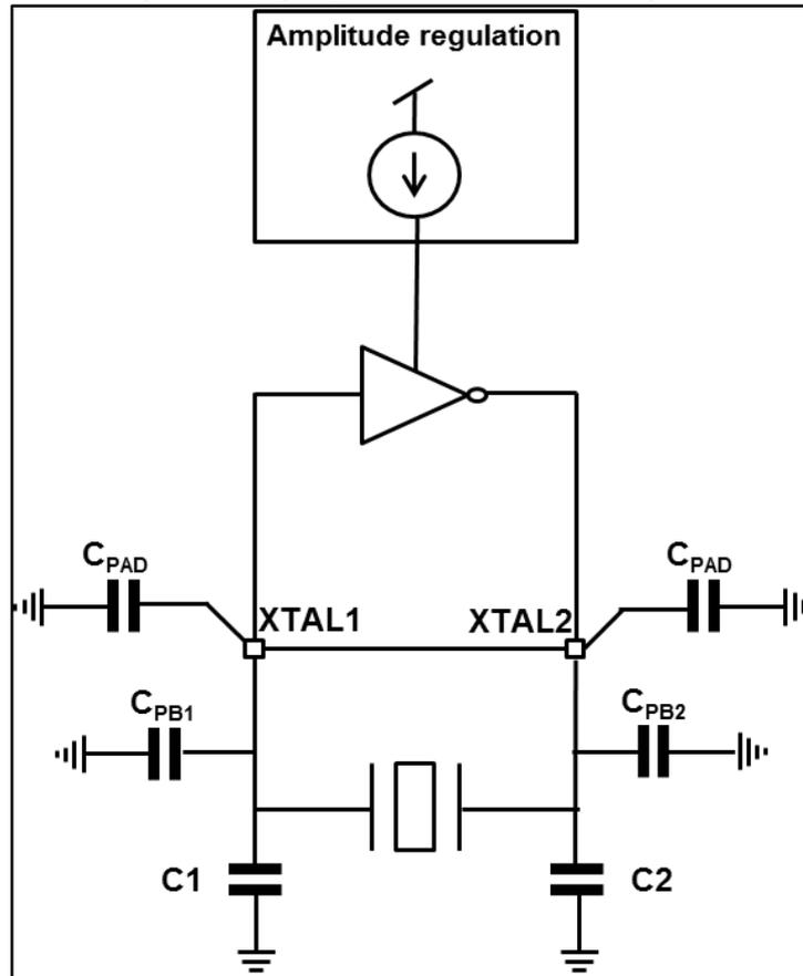
Low power consumption and fast startup time is achieved by choosing a quartz crystal with a low load capacitance  $C_0$ . A reasonable choice for capacitor  $C_0$  is 12 pF. To achieve good frequency stability, the following equation needs to be satisfied:
