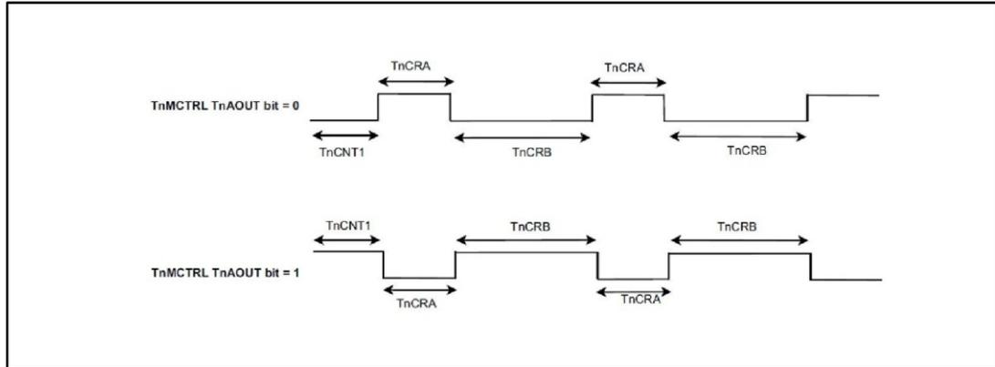
When started the first time, the TnCNT1 starts with value preprogrammed in the register and count down at the clock rate selected by the Timer/Counter 1 clock selector (TnCKC register). When an underflow occurs, the TnCNT1 is reloaded alternatively with TnCRB and TnCRB registers (in this order) and counting proceeds downward from the loaded value.
