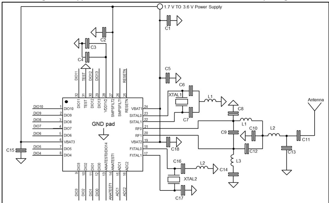
Figure 22: Application circuit: active DC-DC converter WCSP34 package
