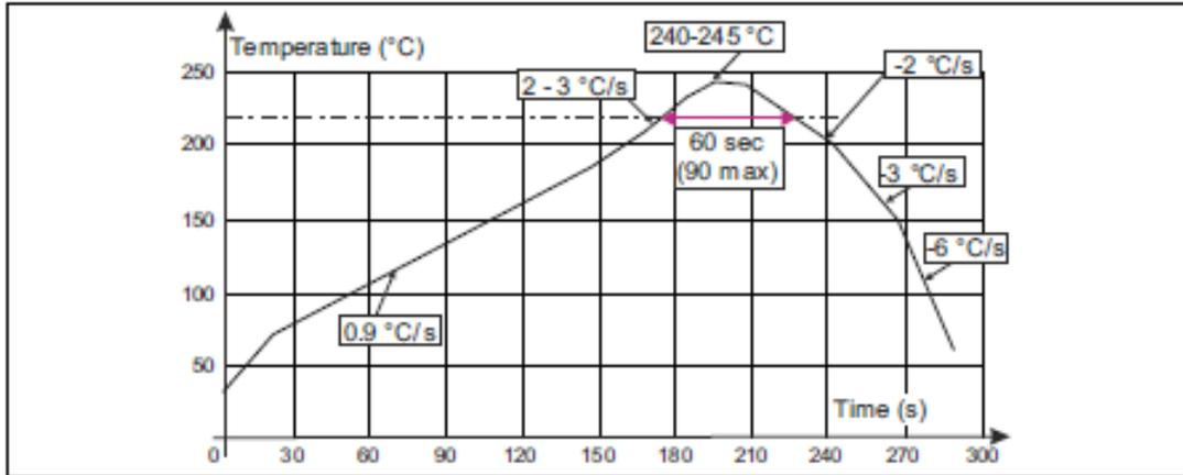
**Table 215: Flip Chip CSP (2.71 x 2.58 x 0.5 pitch 0.4 mm) package reflow profile recommendation**
