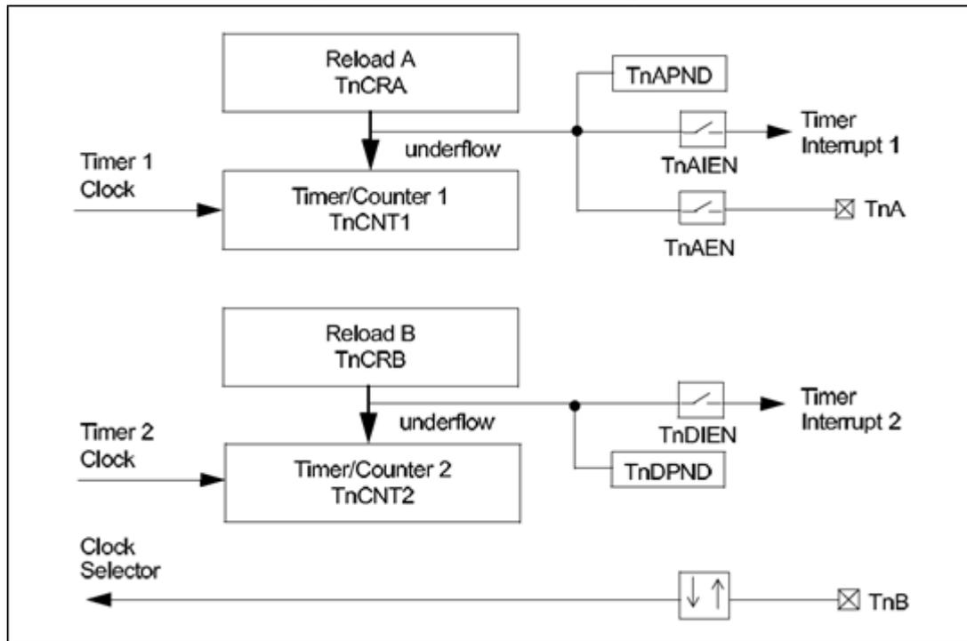
In Mode 3, the timer/counter is configured to operate as a dual independent system timer or dual external-event counter. In addition, Timer/Counter 1 can generate a 50% duty cycle PWM signal on the TnA pin. The TnB pin can be used as an external-event input or pulse-accumulate input, and serve as the clock source to either Timer/Counter 1 or Timer/Counter 2. Both counters can also be operated from the prescaled system clock.
