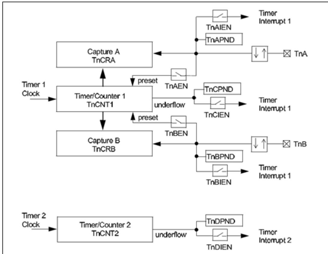
The input signal on TnA and TnB must have a pulse width equal to or greater than one system clock cycle. The values captured in the TnCRB register at different times reflect the elapsed time between transitions on the TnA pin. The same is true for the TnCRB register and TnB pin. Each input pin can be configured to sense either positive-going or negative-going transitions.
