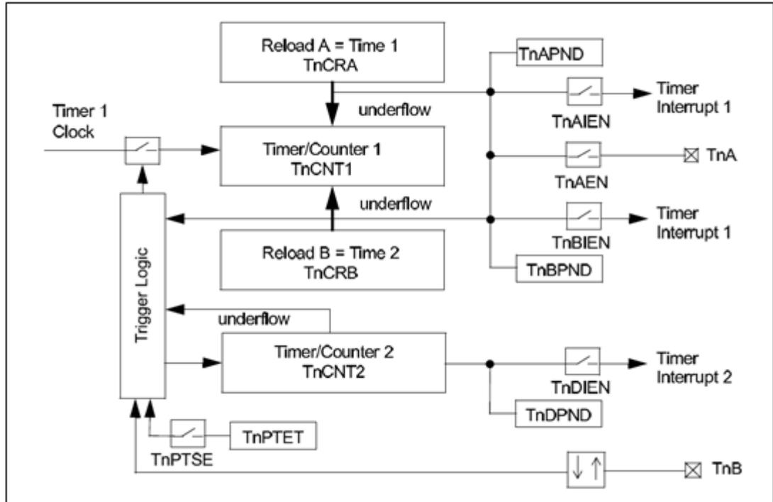
In Mode 1a, Timer/Counter 2 (TnCNT2) behaves differently from the way it behaves in modes 1 to 4. If an underflow condition occurs, the counter is preset to 0x0000 and not 0xFFFF.
