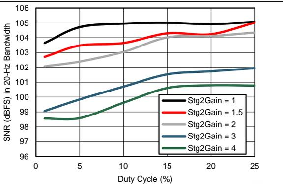
Figure 27. Receiver SNR over Nyquist Bandwidth vs Duty Cycle (Different Stage 2 Gain Settings)
