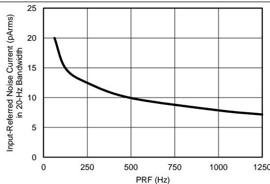
**Figure 22. Receiver Input-Referred Noise in 20-Hz BW in Dynamic Power-Down Mode vs PRF**
