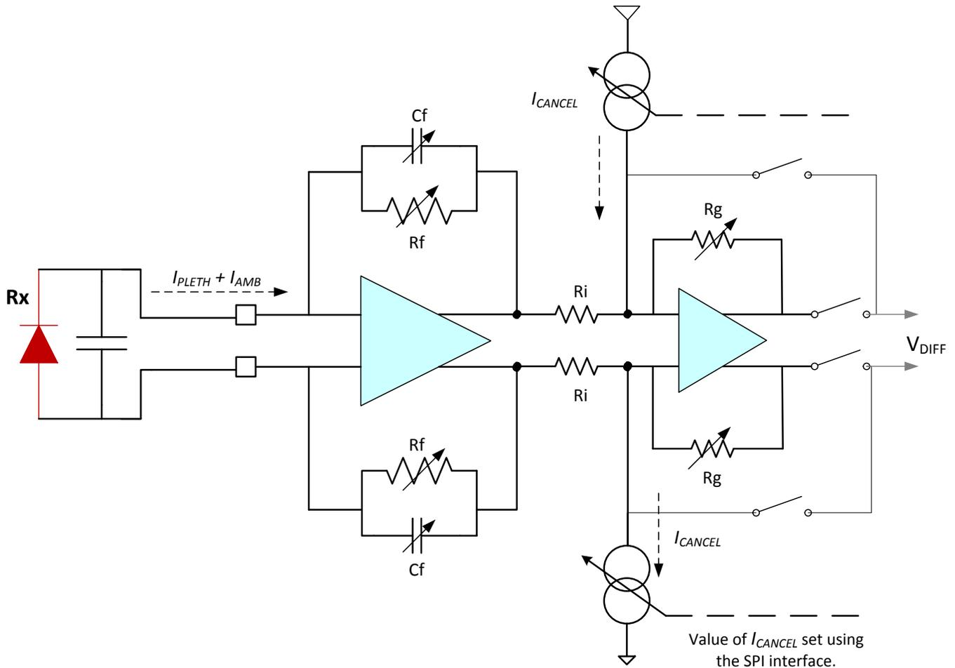
Figure 40. Front-End (I-V Amplifier and Cancellation Stage)
