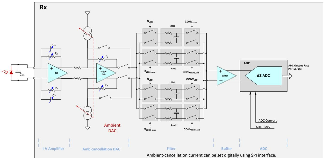
Figure 36. Receiver Front-End
