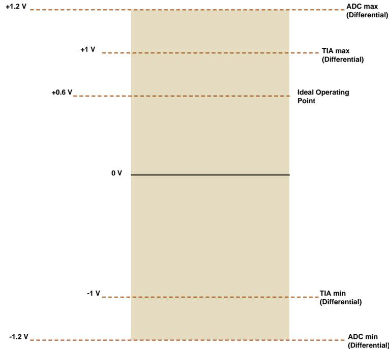
**Figure 38. Signal Levels in TIA and ADC**
