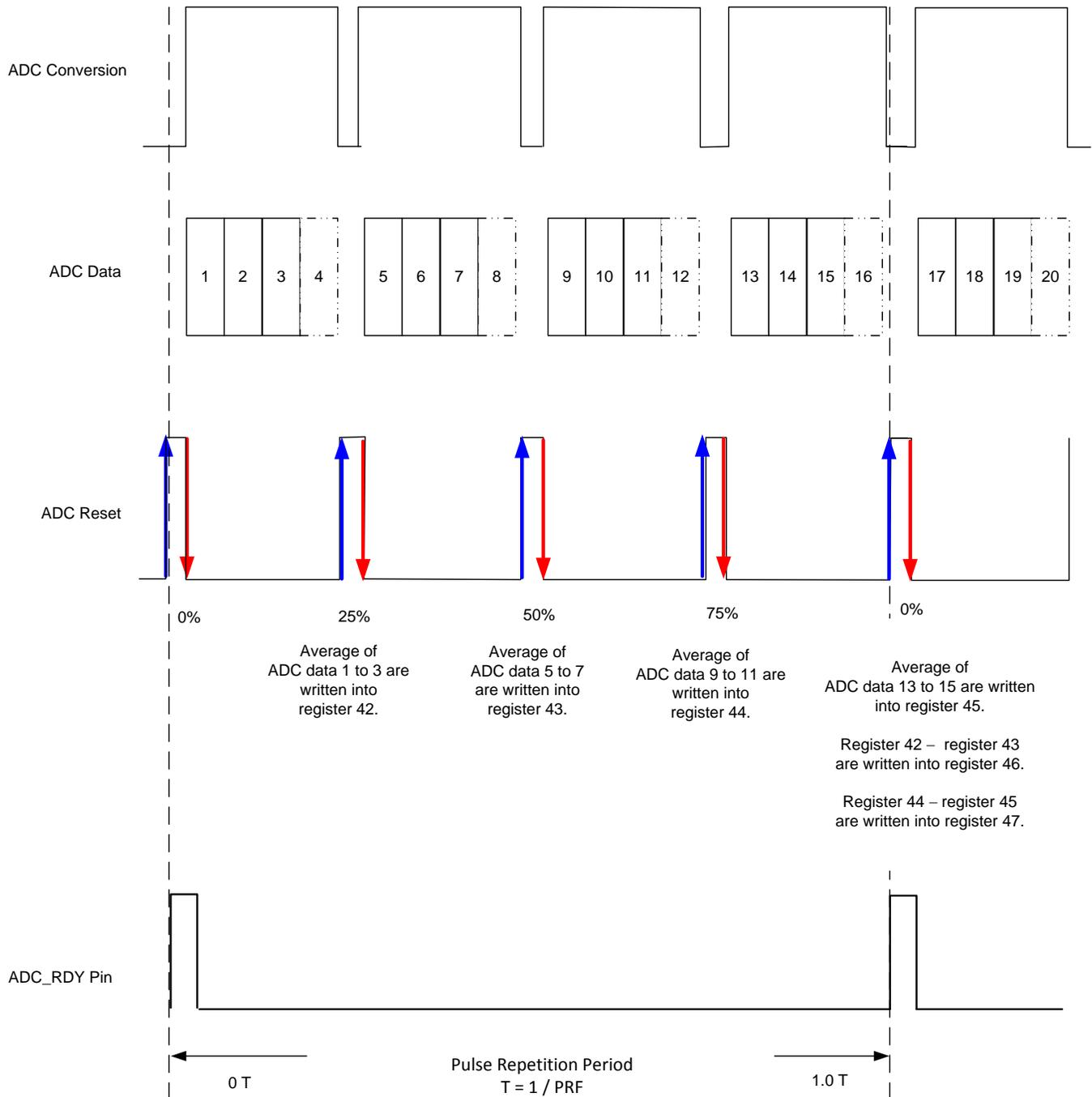
NOTE: Example is with three averages. The value of the NUMAVG[7:0] register bits = 2.
