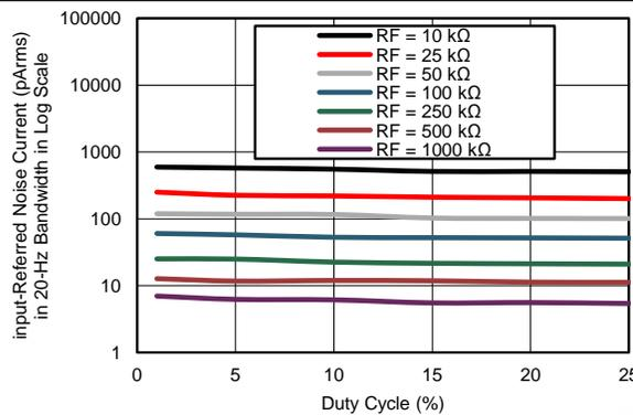
Figure 16. Receiver Input-Referred Noise Current in 20-Hz BW vs Duty Cycle (Different Gain Settings)
