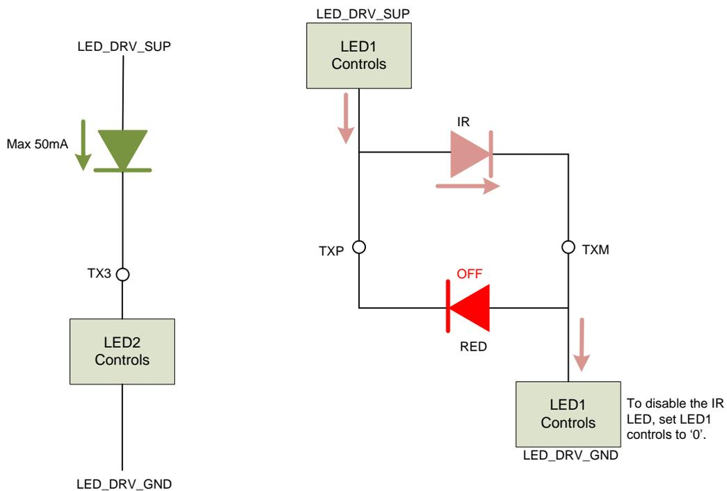
**Figure 59. HRM Application Using the Third LED**
