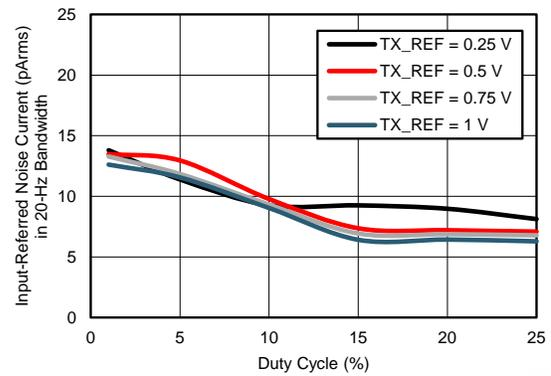
Figure 32. Input Referred Noise Current in 20-Hz BW vs Duty Cycle (TX\_REF Voltage with Tx-Rx Loopback)
