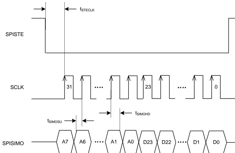
**Figure 2. Serial Interface Timing Diagram, Write Operation**
