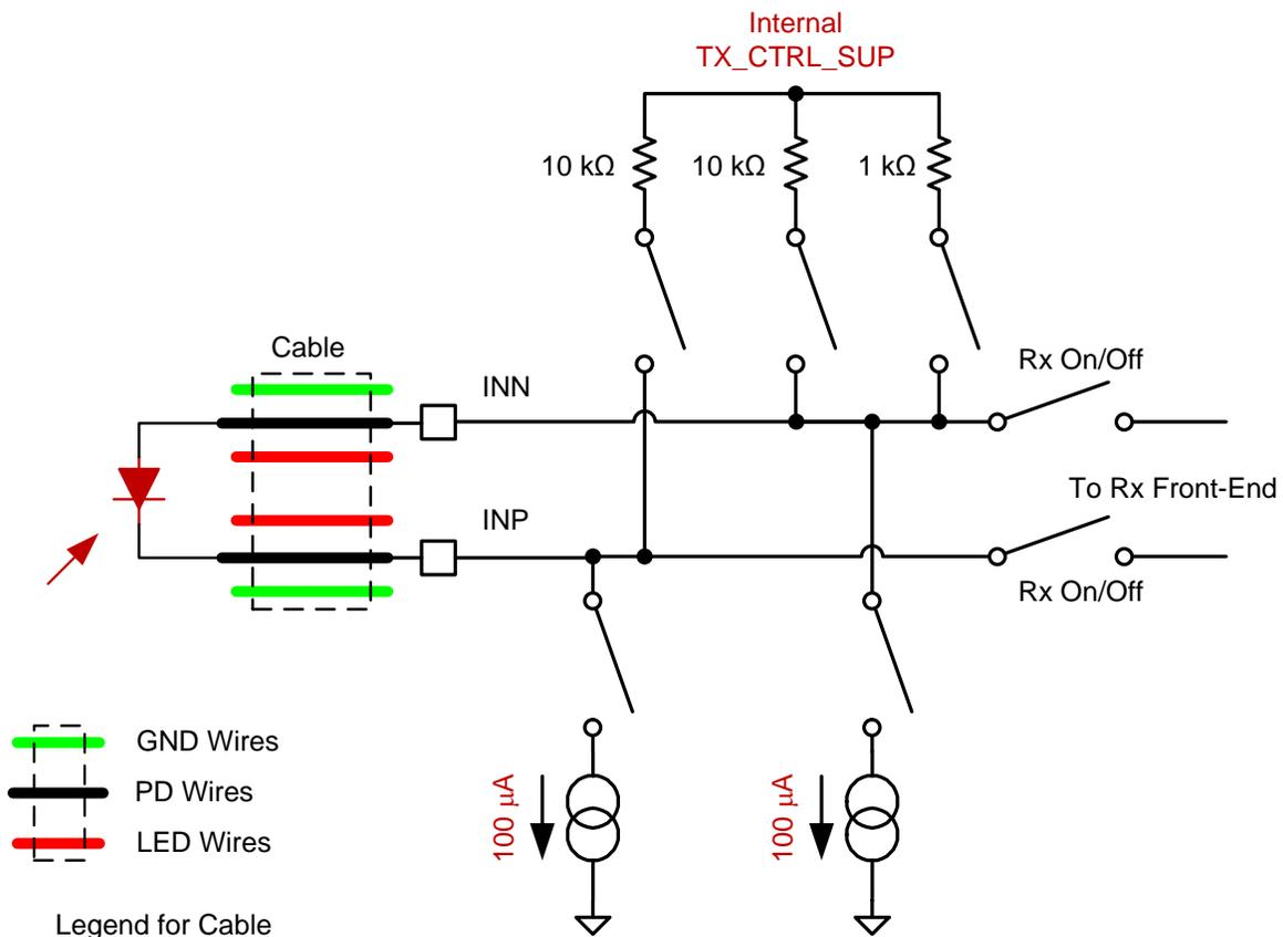
Figure 68. Photodiode Diagnostic
