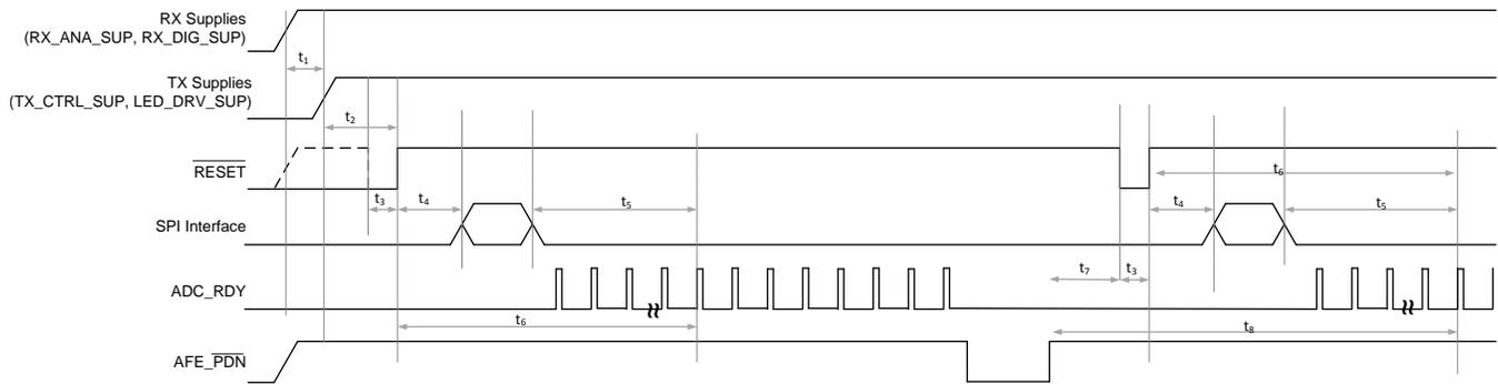
**Figure 3. Supply Ramp and Hardware Power-Down Timing**
