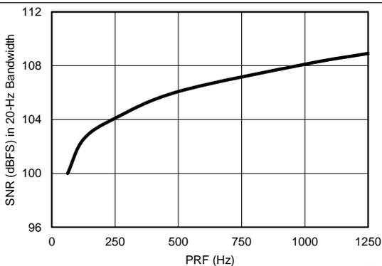
**Figure 21. Receiver SNR in 20-Hz BW in Dynamic Power-Down Mode vs PRF**
