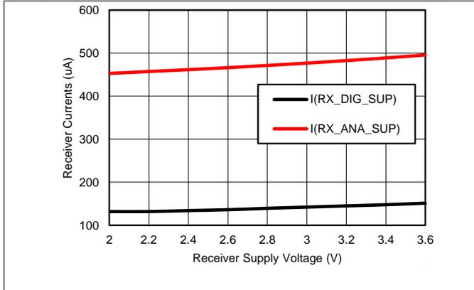
**Figure 5. Receiver Currents vs Receiver Supply Voltage**
