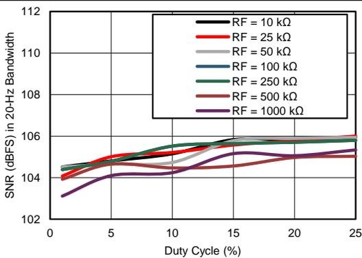
Figure 15. Receiver SNR in 20-Hz BW vs Duty Cycle (Different Gain Settings)
