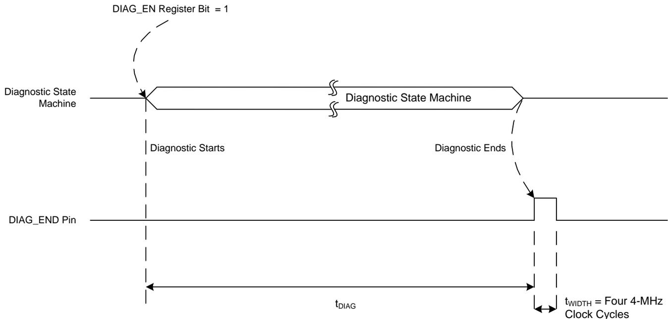
Figure 70. Diagnostic Timing Diagram
