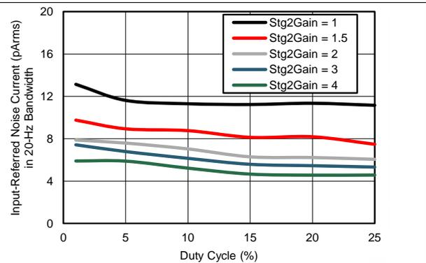
Figure 28. Receiver Input-Referred Noise Current over Nyquist Bandwidth vs Duty Cycle (Different Stage 2 Gain Settings)
