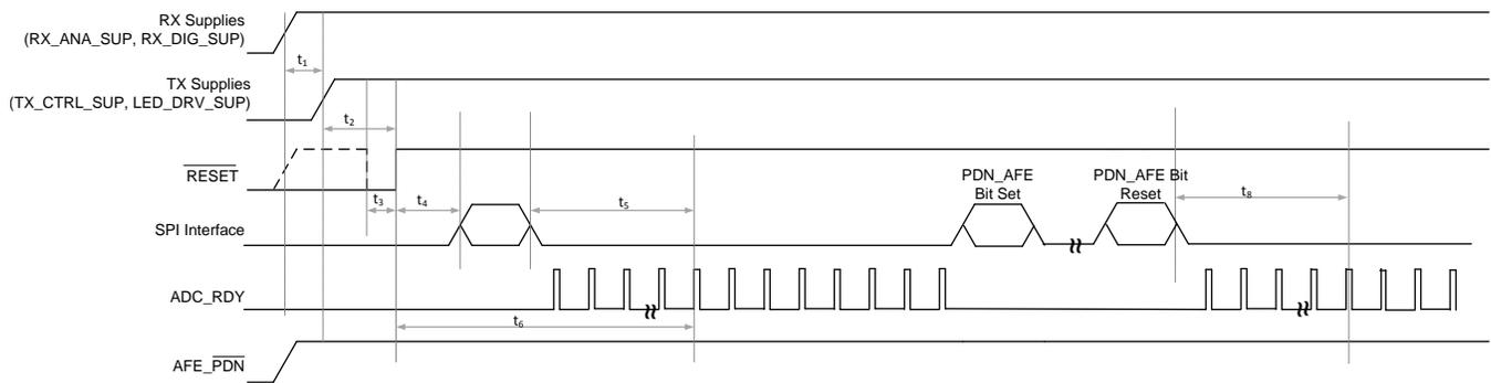
**Figure 4. Supply Ramp and Software Power-Down Timing**
