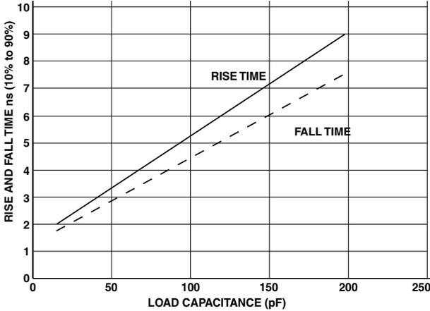
Figure 46. Typical Rise and Fall Times (10% to 90%) vs. Load Capacitance for Driver B at  $V_{DDEXT} = 3.65\text{ V (MAX)}$
