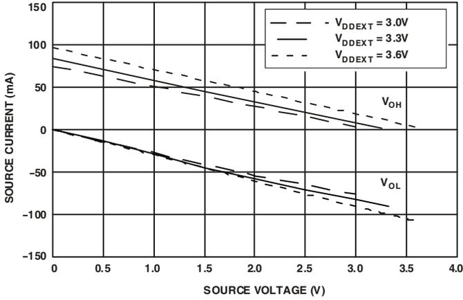
Figure 37. Drive Current D (High  $V_{DDEXT}$ )
