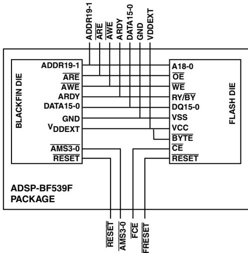
Figure 4. Internal Connection of Flash Memory (ADSP-BF539F)
