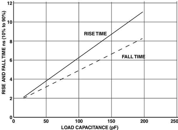
Figure 45. Typical Rise and Fall Times (10% to 90%) vs. Load Capacitance for Driver B at  $V_{DDEXT} = 2.7\text{ V (MIN)}$
