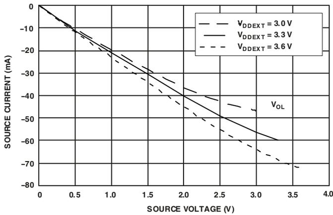
Figure 39. Drive Current E (High  $V_{DDEXT}$ )
