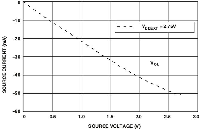
Figure 38. Drive Current E (Low  $V_{DDEXT}$ )
