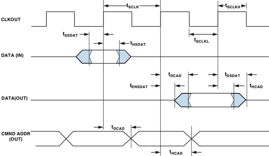
NOTE: COMMAND =  $\overline{SRAS}$ ,  $\overline{SCAS}$ ,  $\overline{SWE}$ ,  $\overline{SDQM}$ ,  $\overline{SMS}$ , SA10, SCKE.
