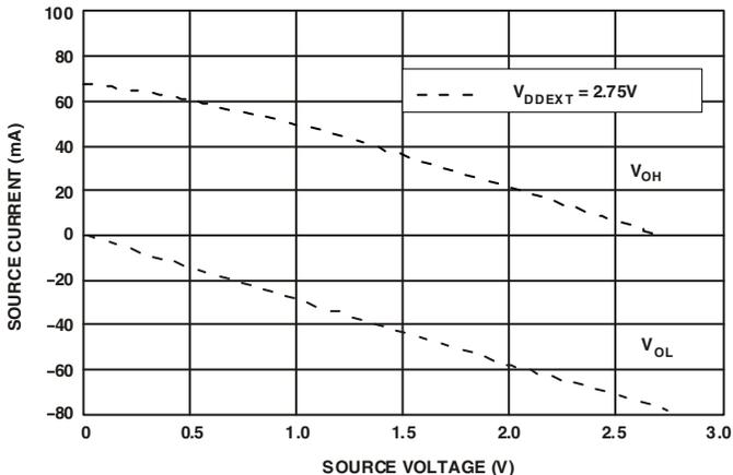
Figure 36. Drive Current D (Low  $V_{DDEXT}$ )
