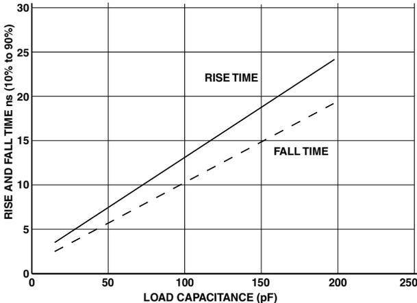
Figure 47. Typical Rise and Fall Times (10% to 90%) vs. Load Capacitance for Driver C at  $V_{DDEXT} = 2.7\text{ V (MIN)}$
