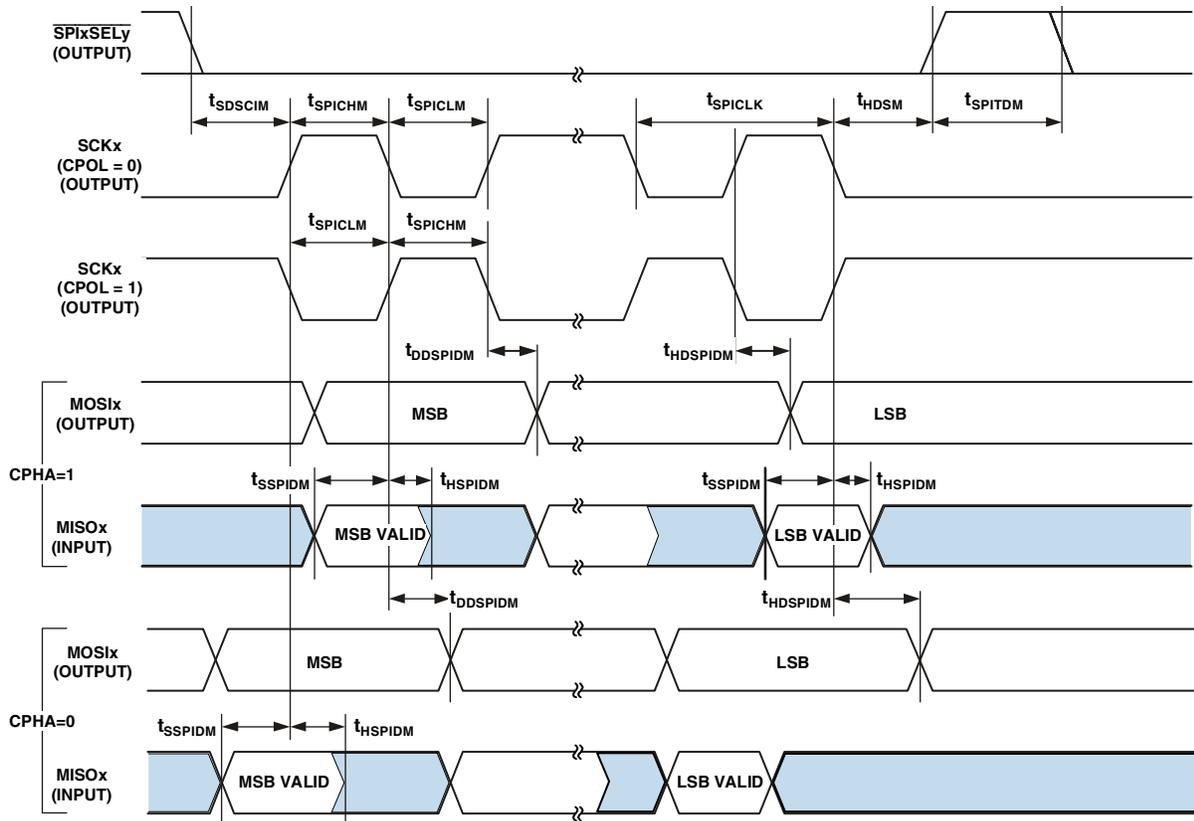
Figure 25. Serial Peripheral Interface (SPI) Ports—Master Timing
