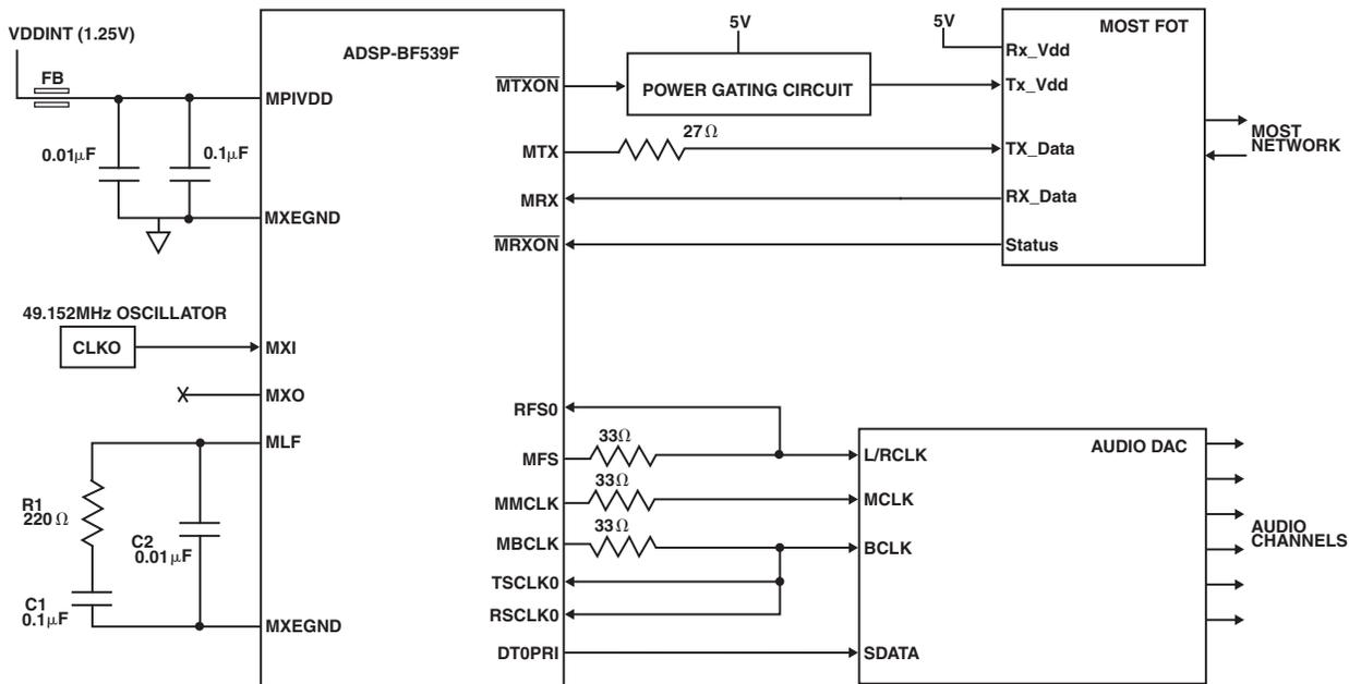
Figure 9. Example Connections of ADSP-BF539/ADSP-BF539F to MOST Network
