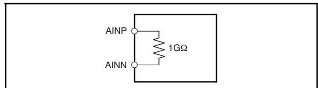
Figure 23. Effective Analog Input Impedances with the Buffer On
