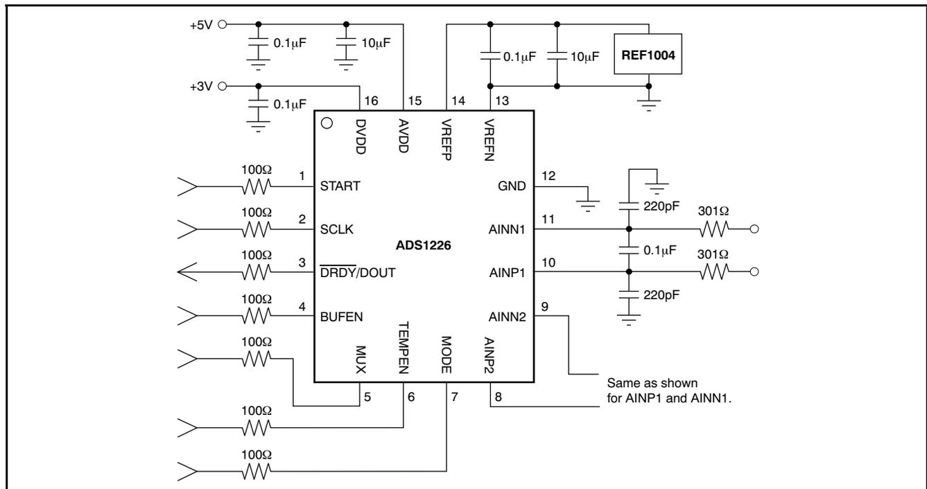
Figure 31. Basic Connections
