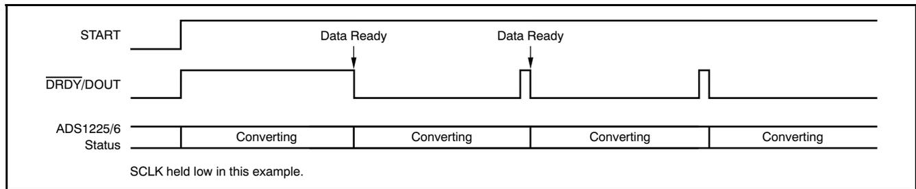
**Figure 27. Conversion with the START Pin Tied High**
