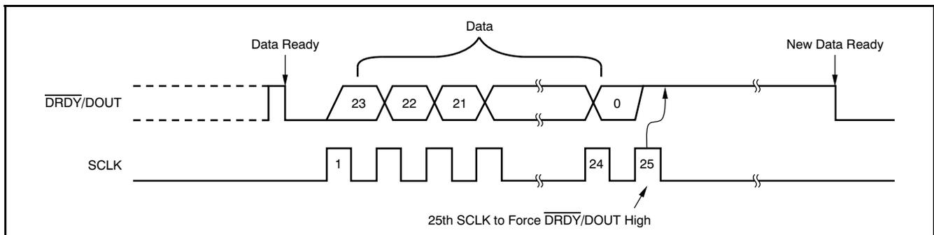
Figure 29. Data Retrieval with  $\overline{\text{DRDY}}/\text{DOUT}$  Forced High Afterwards
