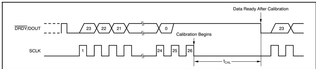
Figure 30. Self-Calibration Timing
