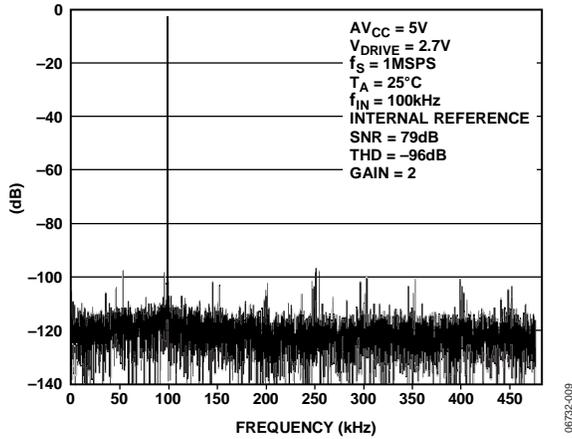
Figure 7. Typical FFT at Gain of 2
