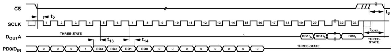
Figure 32. Timing Diagram for a Read Operation with PD0/D<sub>IN</sub> as an Input
