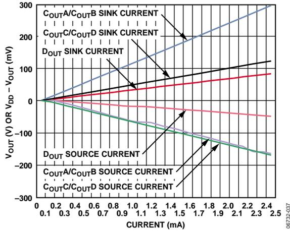
Figure 23. D<sub>OUT</sub> and C<sub>OUT</sub> Source and Sink Current
