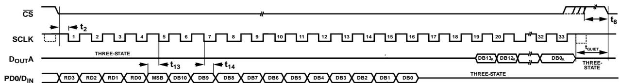
Figure 31. Timing Diagram for Writing to a Register
