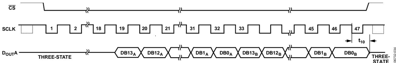
Figure 34. Reading Data from Both ADCs on One D<sub>OUT</sub> Line with 47 SCLK Cycles
