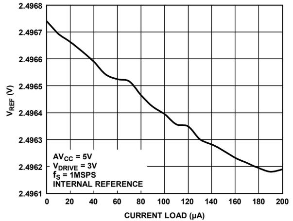
Figure 14.  $V_{REF}$  vs. Reference Output Current Drive
