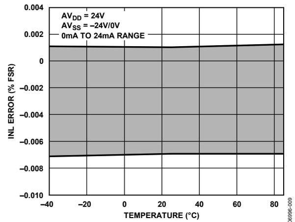
Figure 45. Integral Nonlinearity vs. Temperature, Internal RSET
