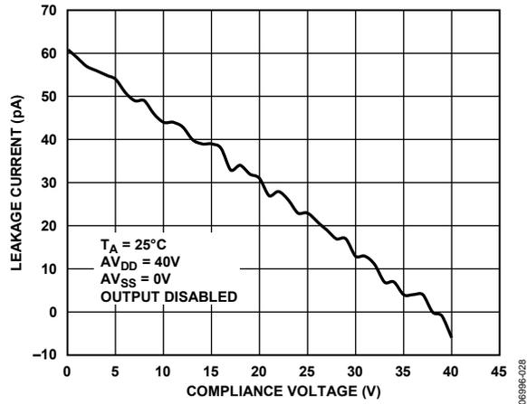
Figure 60. Output Leakage Current vs. Compliance Voltage
