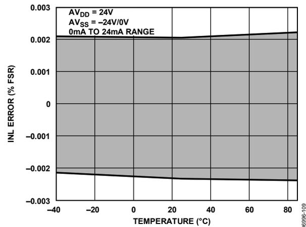
Figure 46. Integral Nonlinearity vs. Temperature, External RSET
