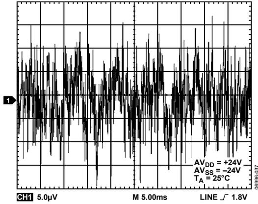
Figure 39. Peak-to-Peak Noise (0.1 Hz to 10 Hz Bandwidth)
