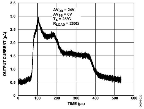
Figure 58. Output Current vs. Time on Power-Up
