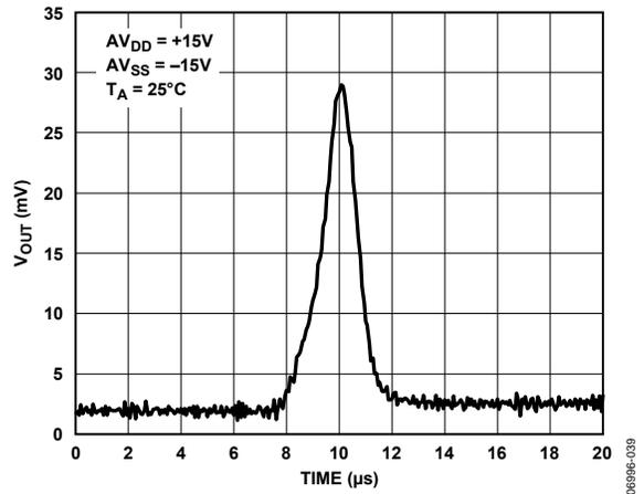
Figure 41. V<sub>OUT</sub> vs. Time on Power-Up
