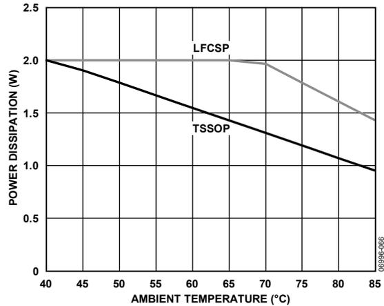
Figure 75. Maximum Power Dissipation vs. Ambient Temperature
