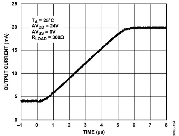
Figure 62. 4 mA to 20 mA Output Current Step
