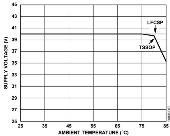
Figure 76. Maximum Supply Voltage vs. Ambient Temperature
