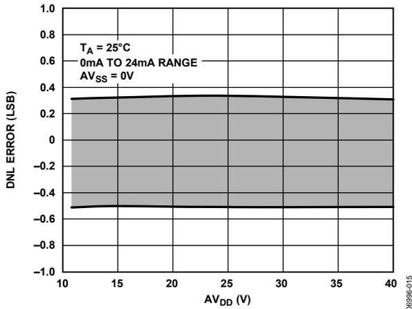
Figure 54. Differential Nonlinearity Error vs.  $AV_{DD}$ , Internal  $R_{SET}$
