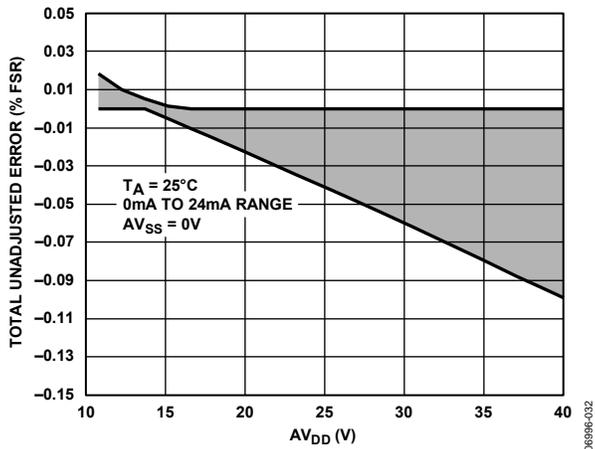
Figure 56. Total Unadjusted Error vs.  $AV_{DD}$ , Internal  $R_{SET}$
