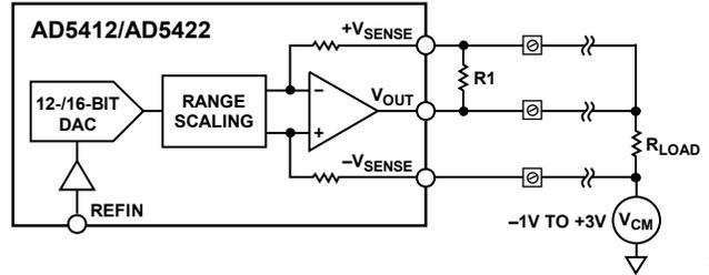
Figure 65. Voltage Output
