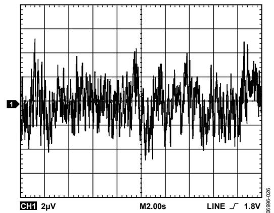
Figure 12. REFOUT Output Noise (0.1 Hz to 10 Hz Bandwidth)
