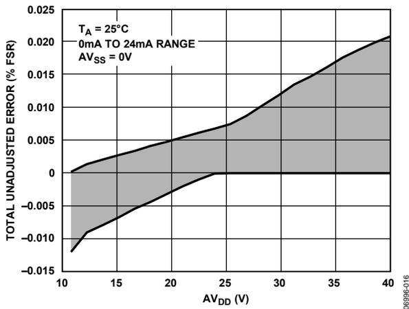
Figure 55. Total Unadjusted Error vs.  $AV_{DD}$ , External  $R_{SET}$
