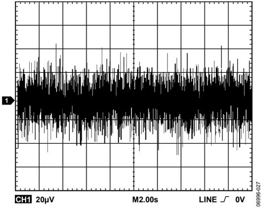
Figure 13. REFOUT Output Noise (100 kHz Bandwidth)
