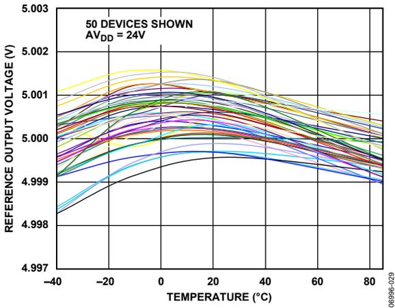
Figure 14. Reference Voltage vs. Temperature
