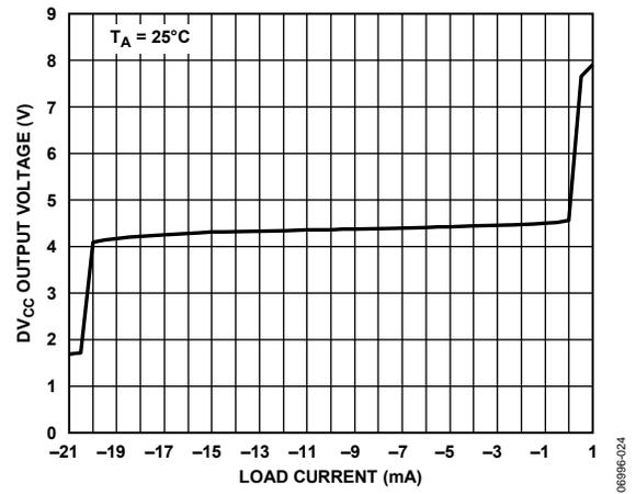
Figure 10.  $DV_{CC}$  Output Voltage vs. Load Current
