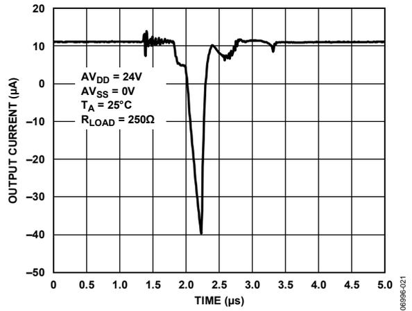
Figure 59. Output Current vs. Time on Output Enable
