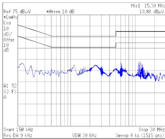
**Figure 4. CE average measurement at 230 V<sub>AC</sub> full load**
