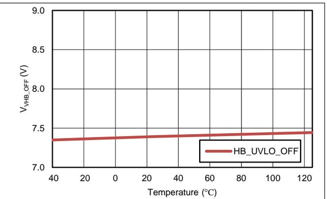
Figure 17. VHB-VHS UVLO Off Threshold vs Temperature
