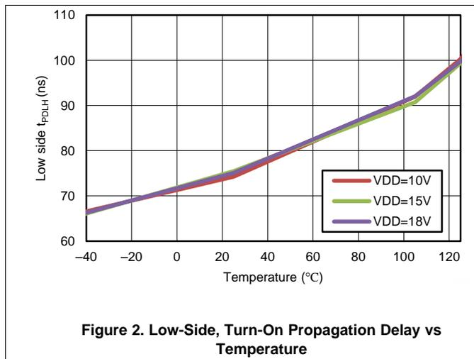
Figure 2. Low-Side, Turn-On Propagation Delay vs Temperature
