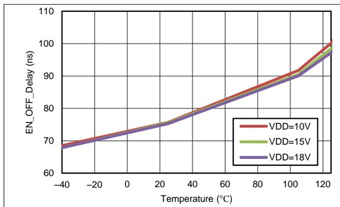
Figure 32. EN OFF Response Time vs Temperature
