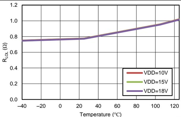
Figure 27. LO Output Pull-Down Resistance vs Temperature
