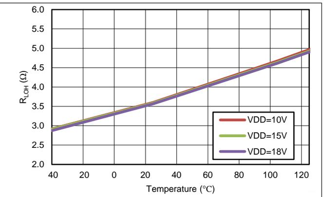
Figure 29. LO Output Pull-Up Resistance vs Temperature
