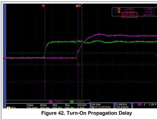
Figure 42. Turn-On Propagation Delay
