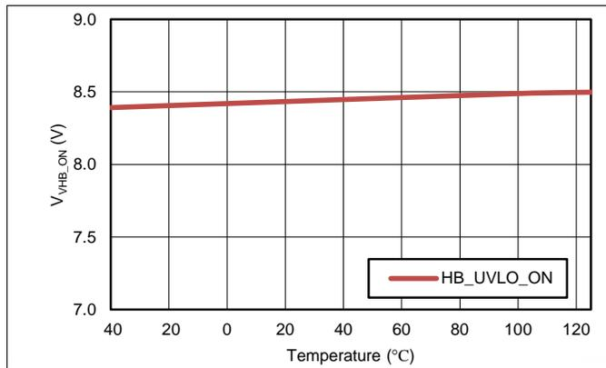
Figure 16. VHB-VHS UVLO On Threshold vs Temperature
