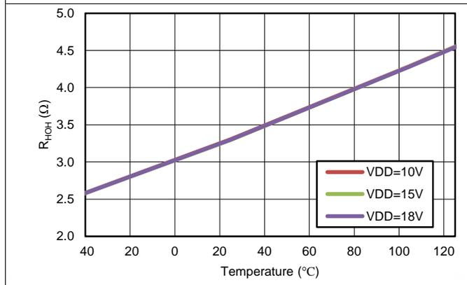
Figure 30. HO Output Pull-Up Resistance vs Temperature
