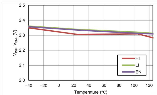
Figure 20. HI/LI/EN Pin High Threshold vs Temperature
