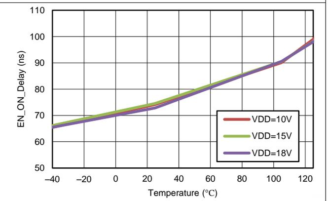
Figure 31. EN ON Response Time vs Temperature
