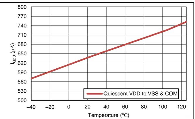
Figure 33. Total Quiescent VDD to VSS and COM Supply Current vs Temperature
