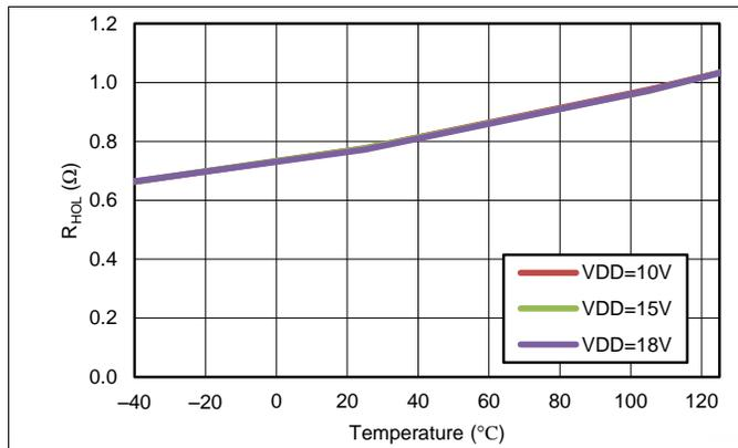
Figure 28. HO Output Pull-Down Resistance vs Temperature
