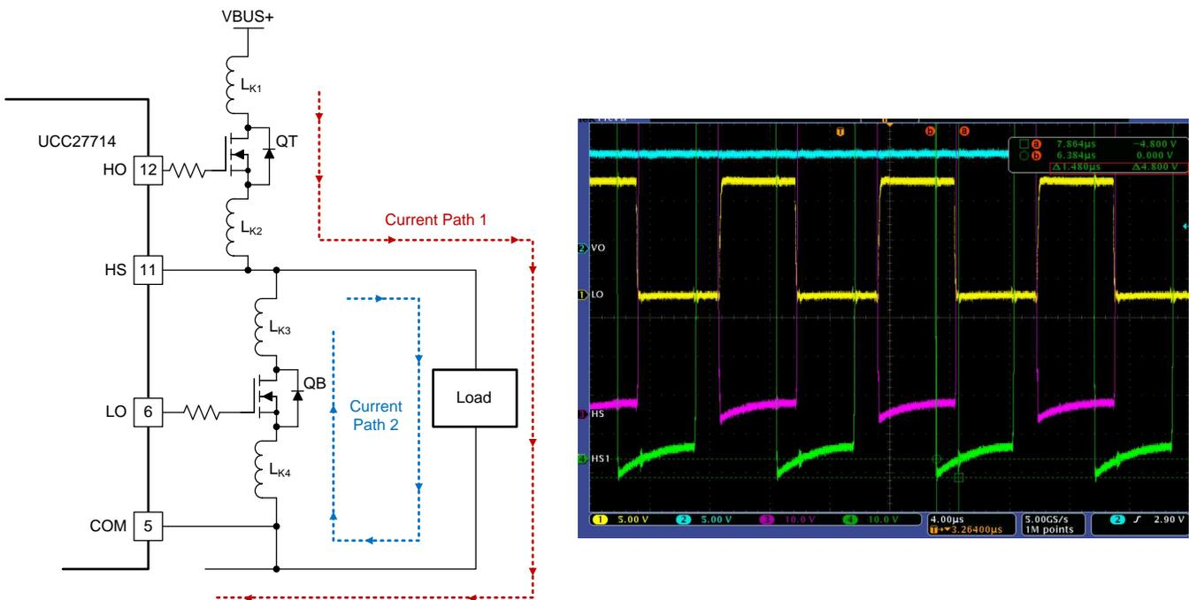
Figure 50. HS Negative Voltage In Half-Bridge Configuration
