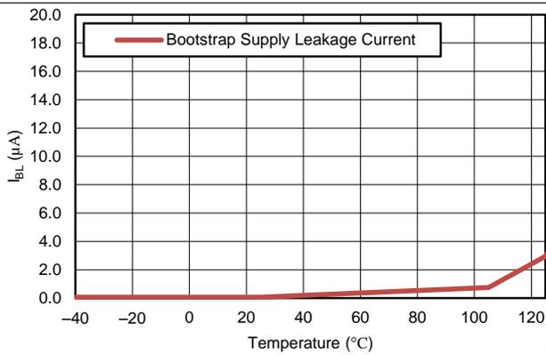
Figure 36. Bootstrap Supply Leakage Current vs Temperature
