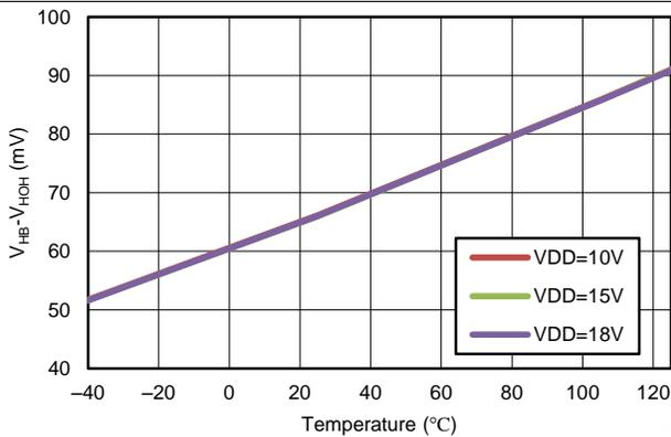
Figure 26. HO Output High Voltage with 20-mA Load vs Temperature
