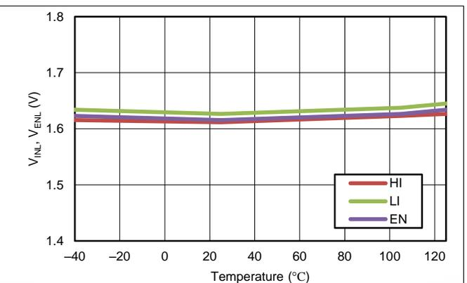
Figure 21. HI/LI/EN Pin Low Threshold vs Temperature
