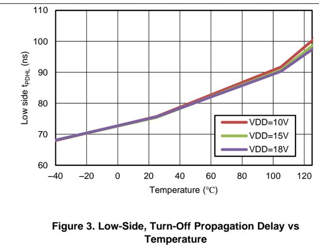
Figure 3. Low-Side, Turn-Off Propagation Delay vs Temperature
