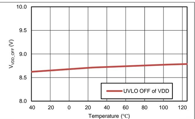
Figure 15. VDD UVLO Off Threshold vs Temperature
