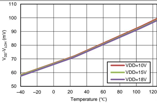
Figure 24. LO Output High Voltage with 20-mA Load vs Temperature
