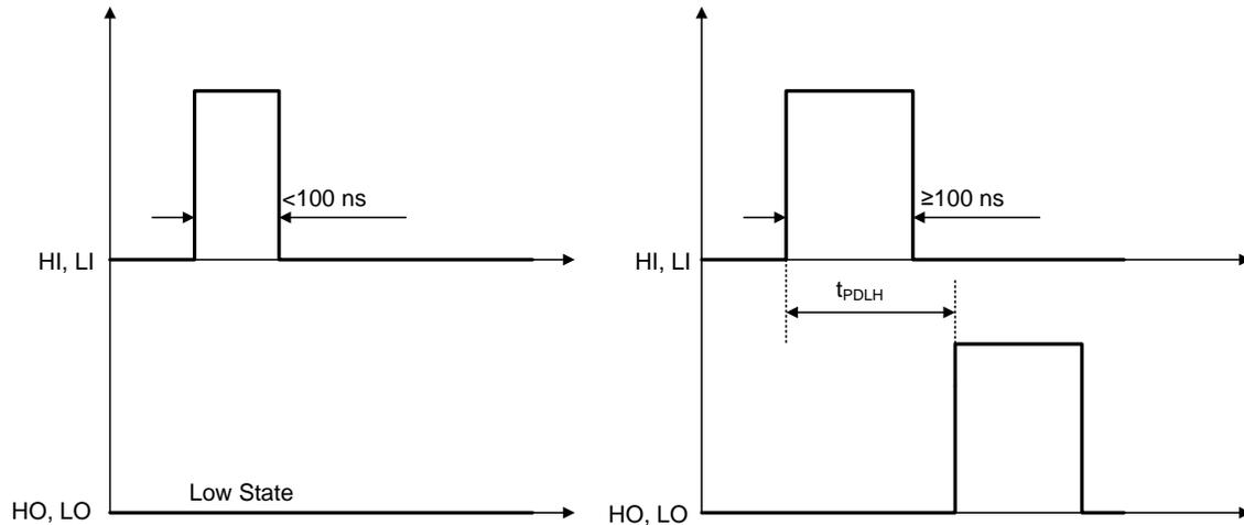
**Figure 46. Minimum Turn-On Pulse**
