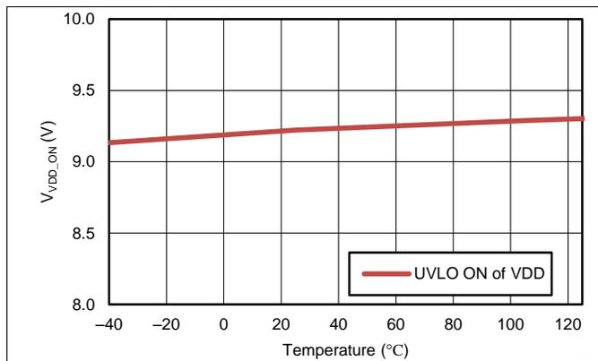
Figure 14. VDD UVLO On Threshold vs Temperature
