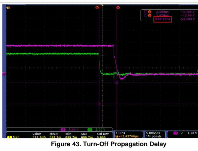
Figure 43. Turn-Off Propagation Delay
