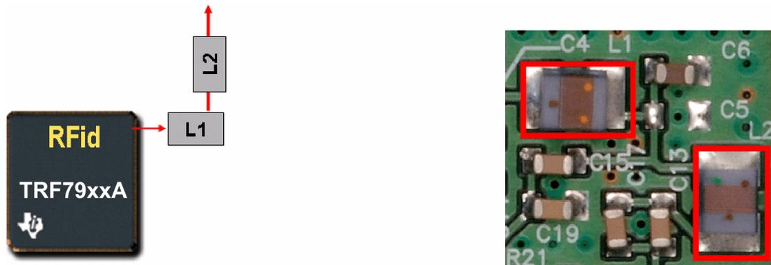
**NOTE:** TI does not recommend using any inductor sizes below 0603, because the output power can be compromised. If smaller inductors are absolutely necessary, it is up to the customer to confirm output performance.
