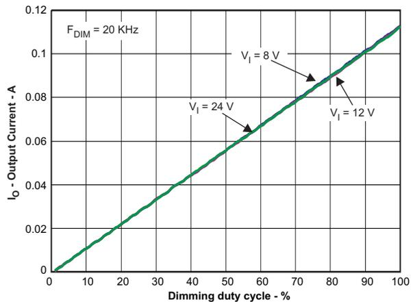
Figure 4. Dimming Linearity
