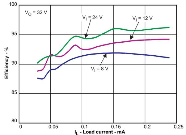
Figure 2. Efficiency vs Load Current by Input Voltage
