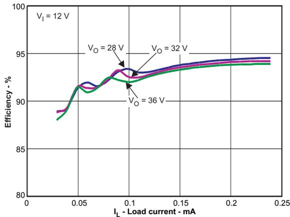
Figure 1. Efficiency vs Load Current by Output Voltage
