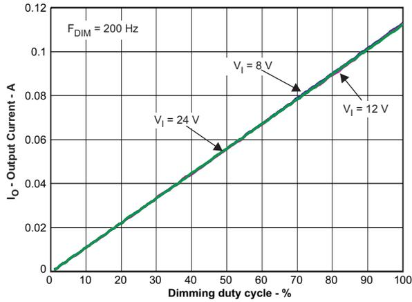
Figure 5. Dimming Linearity
