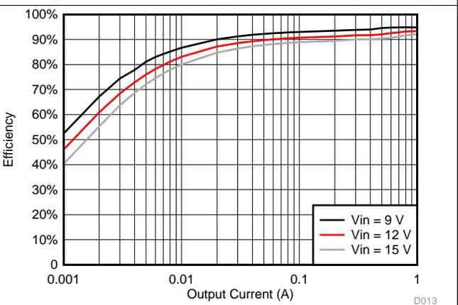
Figure 12. TPS561201  $V_{OUT} = 5\text{ V}$  Efficiency,  $L = 4.7\ \mu\text{H}$
