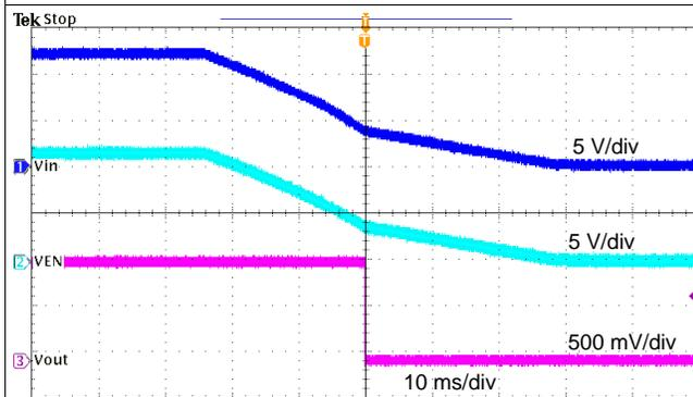
Figure 32. TPS561201 Shutdown Relative to  $V_I$
