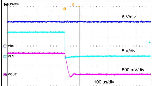
Figure 33. TPS561201 Shutdown Relative to EN
