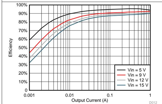
Figure 11. TPS561201  $V_{OUT} = 3.3\text{ V}$  Efficiency,  $L = 3.3\ \mu\text{H}$
