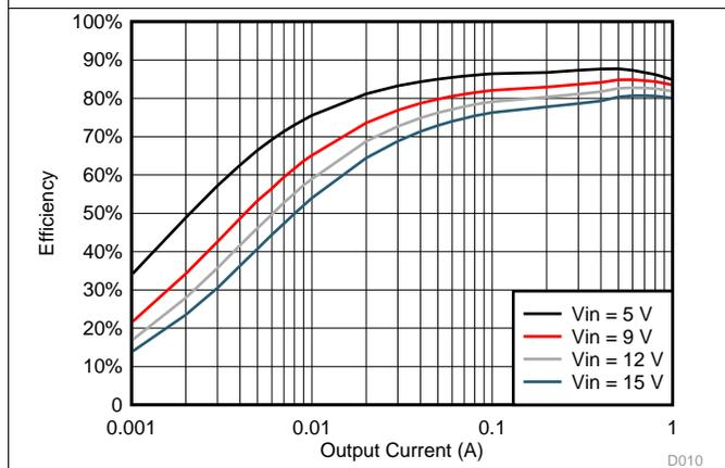
Figure 9. TPS561201  $V_{OUT} = 1.05\text{ V}$  Efficiency,  $L = 2.2\ \mu\text{H}$
