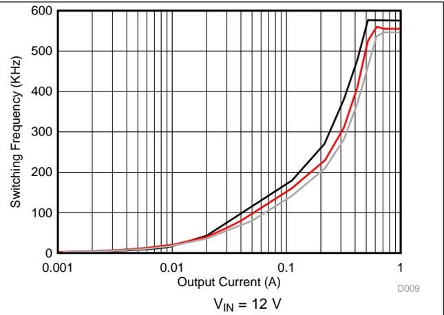
Figure 8. TPS561201 Switching Frequency vs Output Current
