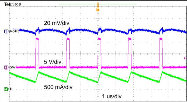
**Figure 25. TPS561201 Output Voltage Ripple,  $I_{OUT} = 1$  A**
