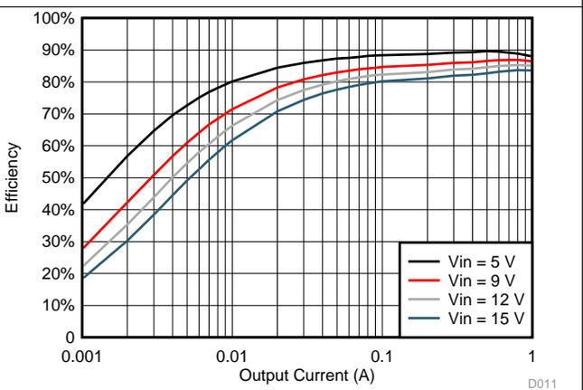
Figure 10. TPS561201  $V_{OUT} = 1.5\text{ V}$  Efficiency,  $L = 2.2\ \mu\text{H}$
