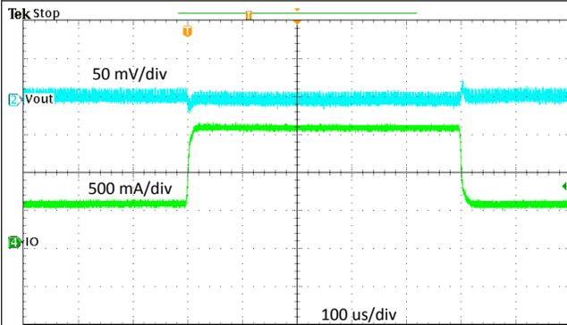
**Figure 28. TPS561201 Transient Response, 0.5 to 1.5 A**
