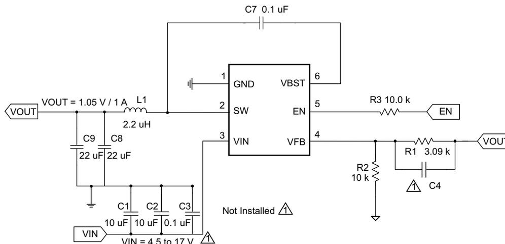
Figure 17. TPS561201 and TPS561208 1.05-V/1-A Reference Design
