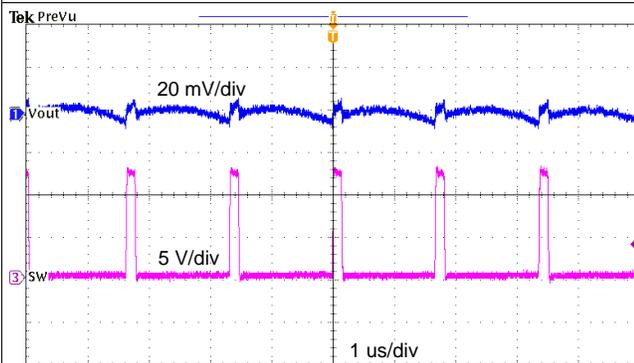
**Figure 26. TPS561208 Output Voltage Ripple,  $I_{OUT} = 0$  A**
