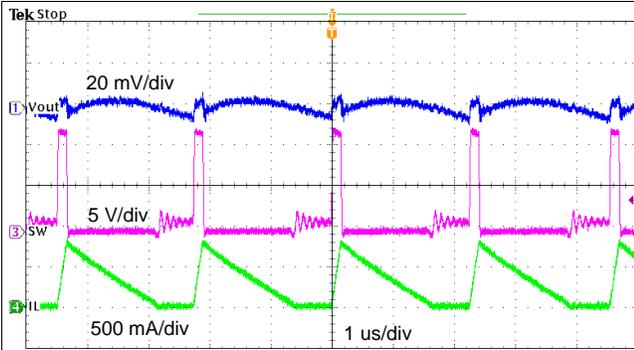
**Figure 24. TPS561201 Output Voltage Ripple,  $I_{OUT} = 0.25$  A**
