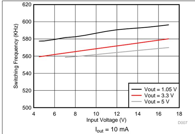
Figure 7. TPS561208 Switching Frequency vs Input Voltage
