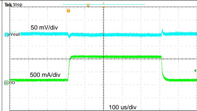
**Figure 29. TPS561208 Transient Response 0.1 to 1 A**
