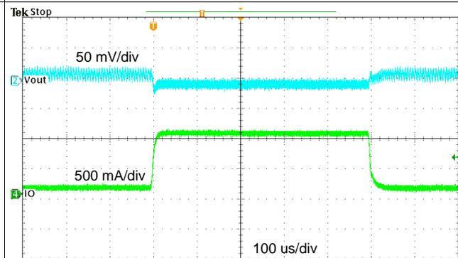
**Figure 27. TPS561201 Transient Response, 0.1 to 1 A**
