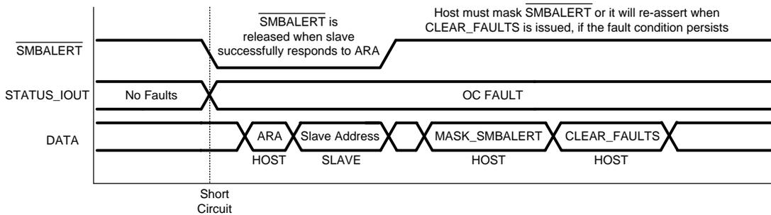
Figure 38. Example Auto ARA Response to Persistent Fault
