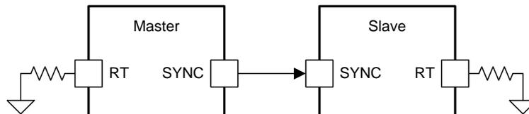
**Figure 27. Master-Slave Synchronization and Phase Interleaving Setting**
