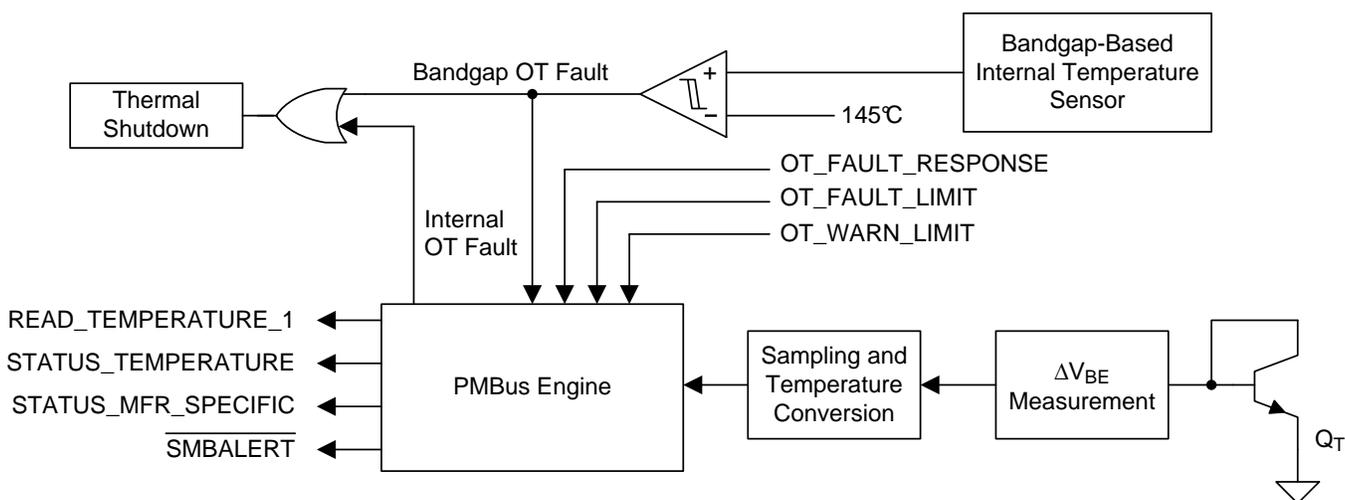
Figure 33. Overtemperature Protection
