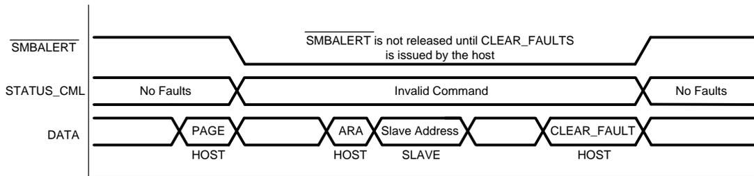
Figure 35. Example Standard ARA Response to Nonpersistent Fault
