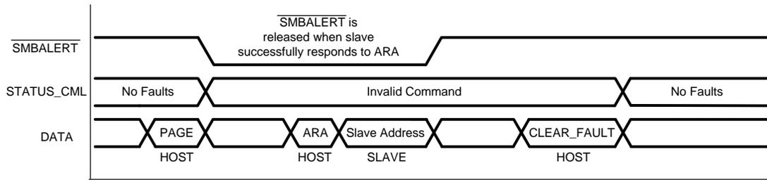
Figure 37. Example Auto ARA Response to Nonpersistent Fault
