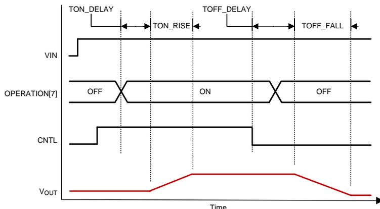
**Figure 24. Turnon Controlled by Both Operation<sup>(1)</sup> and Control<sup>(1)</sup>**
