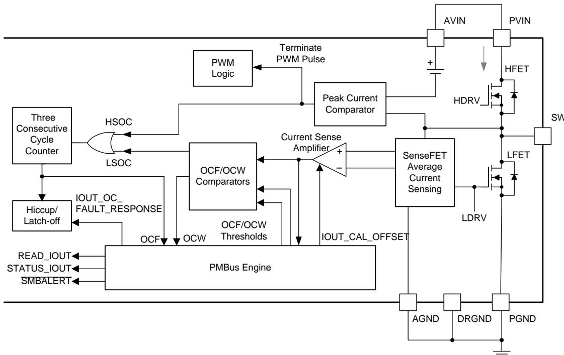
**Figure 32. SenseFET Average Current Sensing and Overcurrent Protection**
