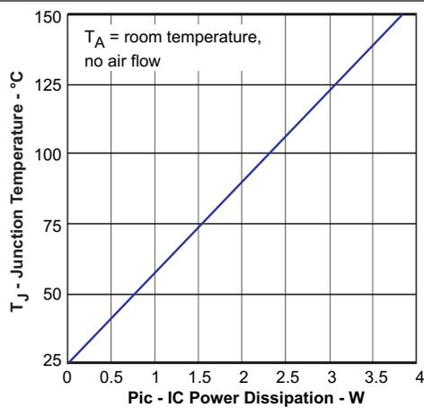
Figure 42. Junction Temperature vs IC Power Dissipation
