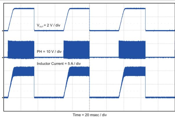
Figure 45. Hiccup Mode Current Limit
