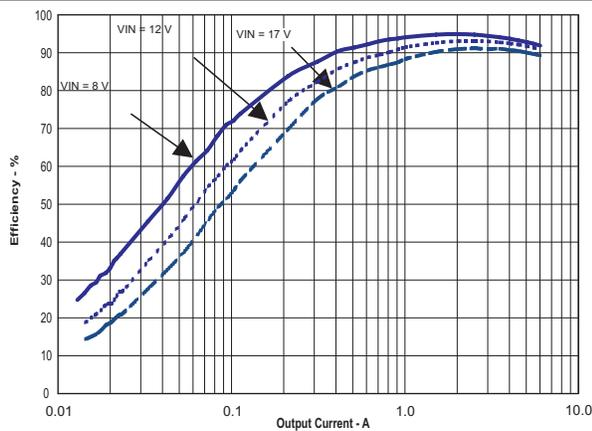
Figure 44. Efficiency vs Load Current
