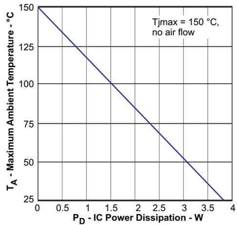
Figure 41. Maximum Ambient Temperature vs IC Power Dissipation
