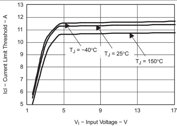
Figure 13. High-Side Current Limit Threshold vs Input Voltage
