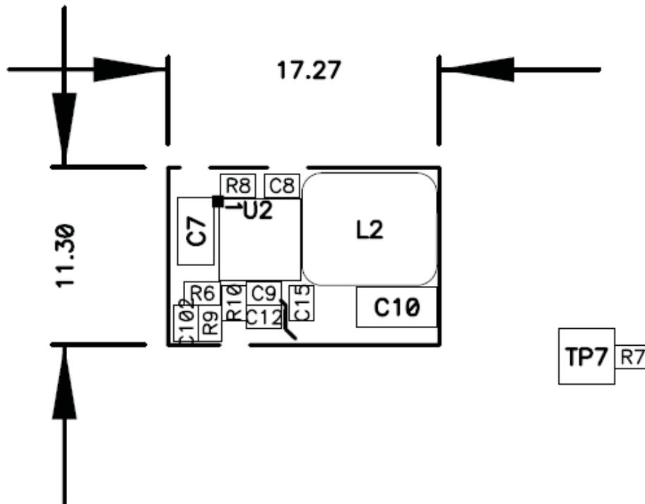
Figure 47. Ultra-Small PCB Layout Using TPS54622 (PMP4854-2)
