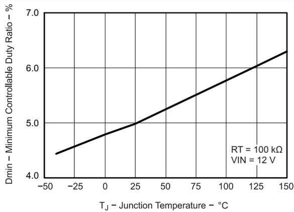
Figure 15. Minimum Controllable Duty Ratio vs Junction Temperature
