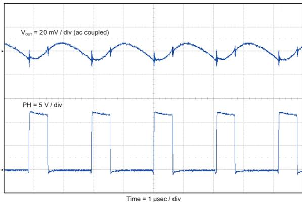
Figure 34. Output Voltage Ripple With No Load
