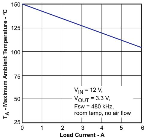
Figure 40. Maximum Ambient Temperature vs Load Current
