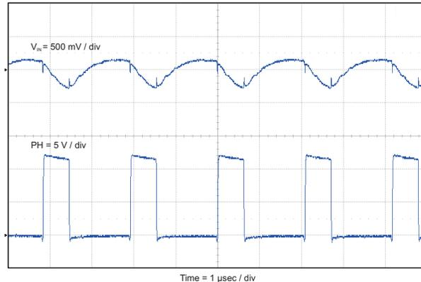
Figure 35. Input Voltage Ripple With Full Load
