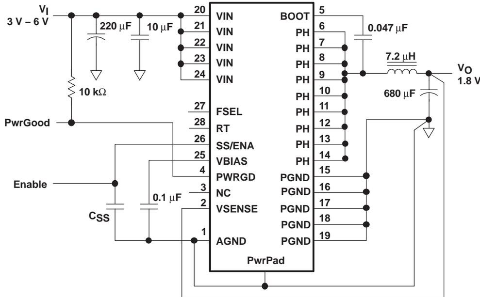
Figure 10. Application Circuit
